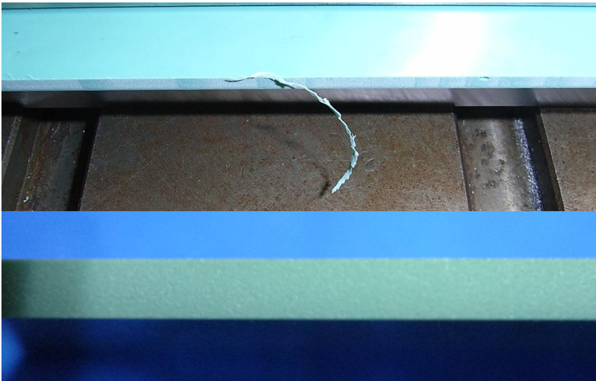
Fig. 2.3.10 Cutting surface by worn endmill
