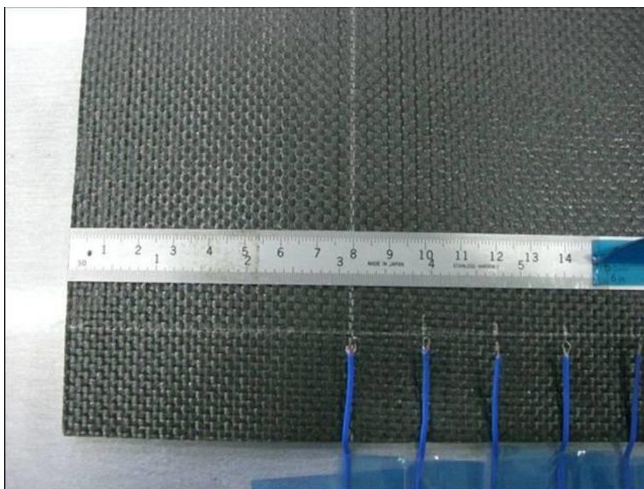
Fig. 3.4.4 Burring process of K type thermocouple
