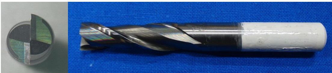
Fig. 3.2.7 Painted uncoated cemented carbide solid endmill
