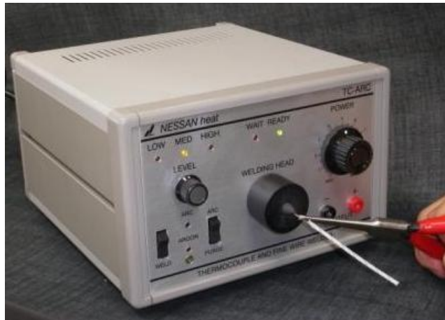
Fig. 3.4.2 Thermocouple welding equipment
