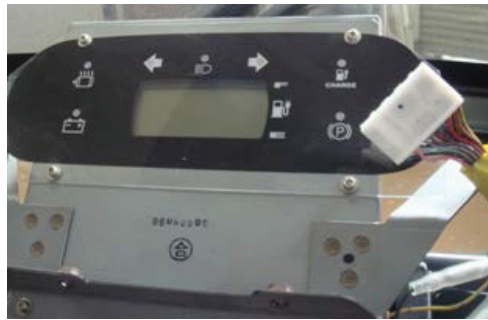
Fig. 2.3.8 Vehicle ECU
