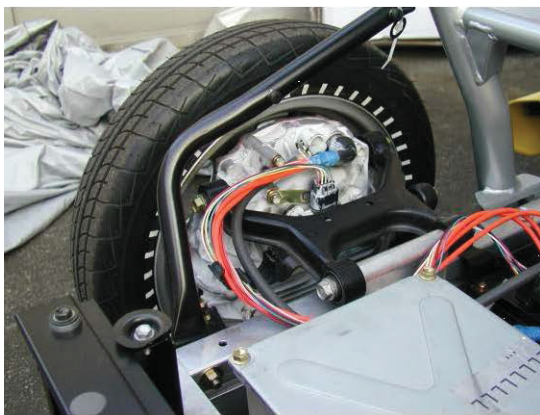
Fig. 2.3.3 In-wheel motor
