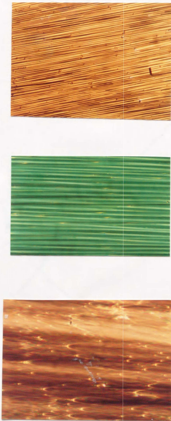
Fig.17. The polarizing microscope pictures of the smectic A structure of 764E. (a), (b) and (c) show the results for the samples of 1.8\mu\text{m} , 8\mu\text{m} and 20\mu\text{m} , respectively.
