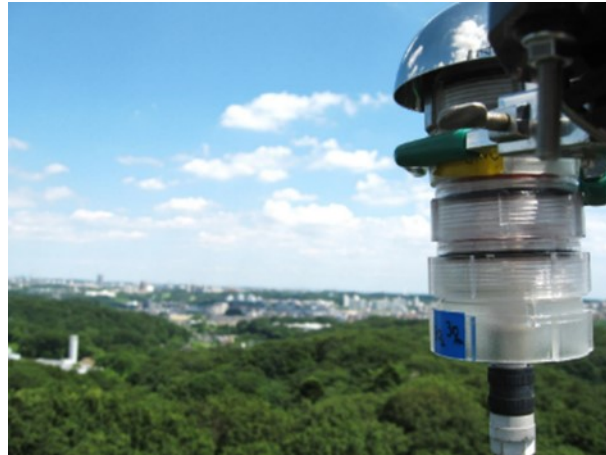
Fig. 2-5. Photo of filter-pack holder at the 30 m of the tower
