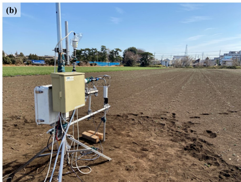
Fig. 4-2. Photo of the REA sampling system in (a) soybean-growing and (b) fallow periods.
