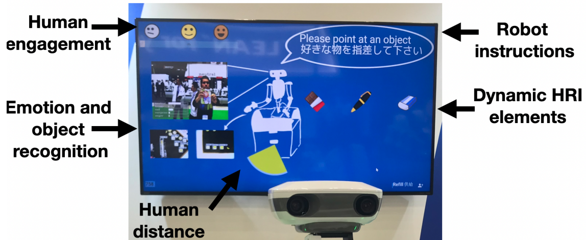
Figure 3.2: Main elements of the designed Graphical User Interface (GUI)
