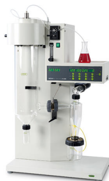
Fig. 1-15 Appearance of a spray dryer (Mini Spray Dryer B-290, Nihon BUCHI K.K.).
