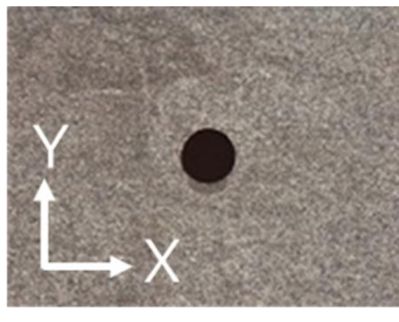
Fig.6.8. The artificial keyhole with a 0.940 mm depth, a 0.317 mm MDXD, and a 0.316 mm MDYD as true values.
