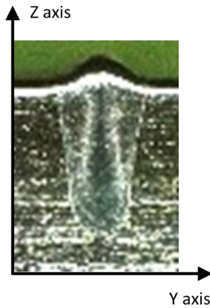
Fig. 6.7. A metallographic cross-section image of the keyhole
