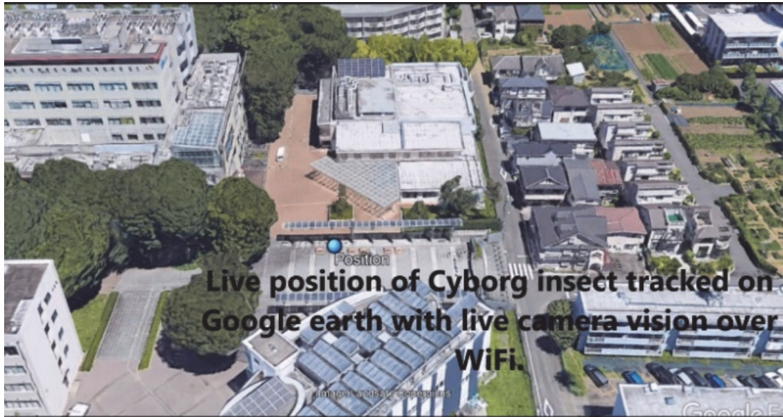
Figure 14: Live GPS map relayed onto Google earth using the WiFi enable CameraRoach system.
