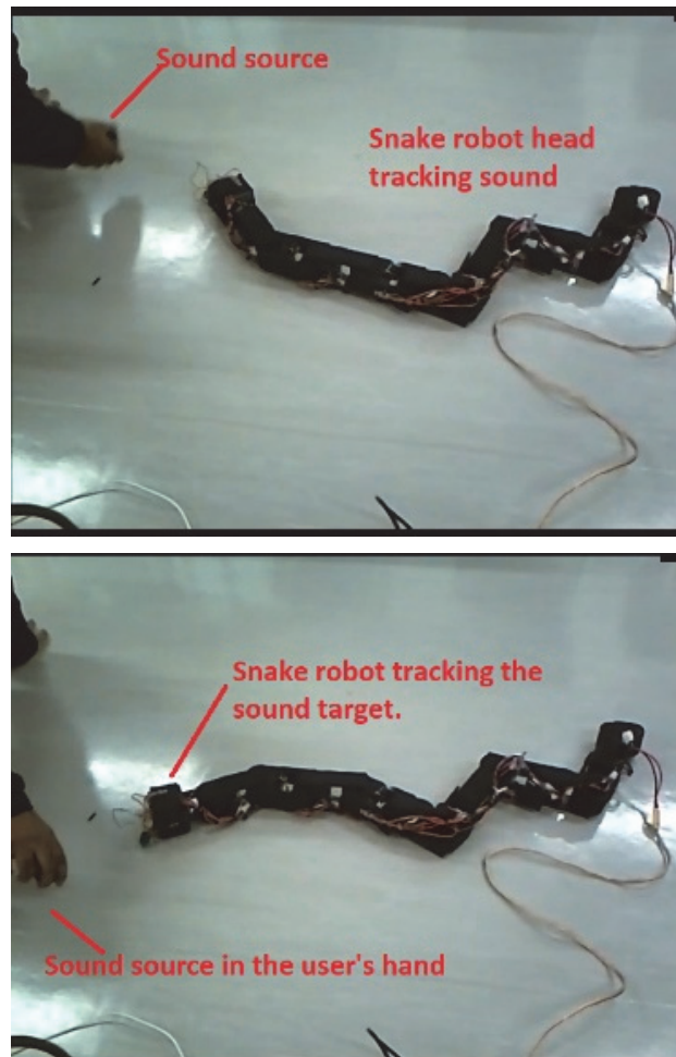
Figure 7: Snake robot first half of the body tracking the sound source in user’s hand. The sound source is a Bluetooth speaker playing a sinusoidal sound waveform.
