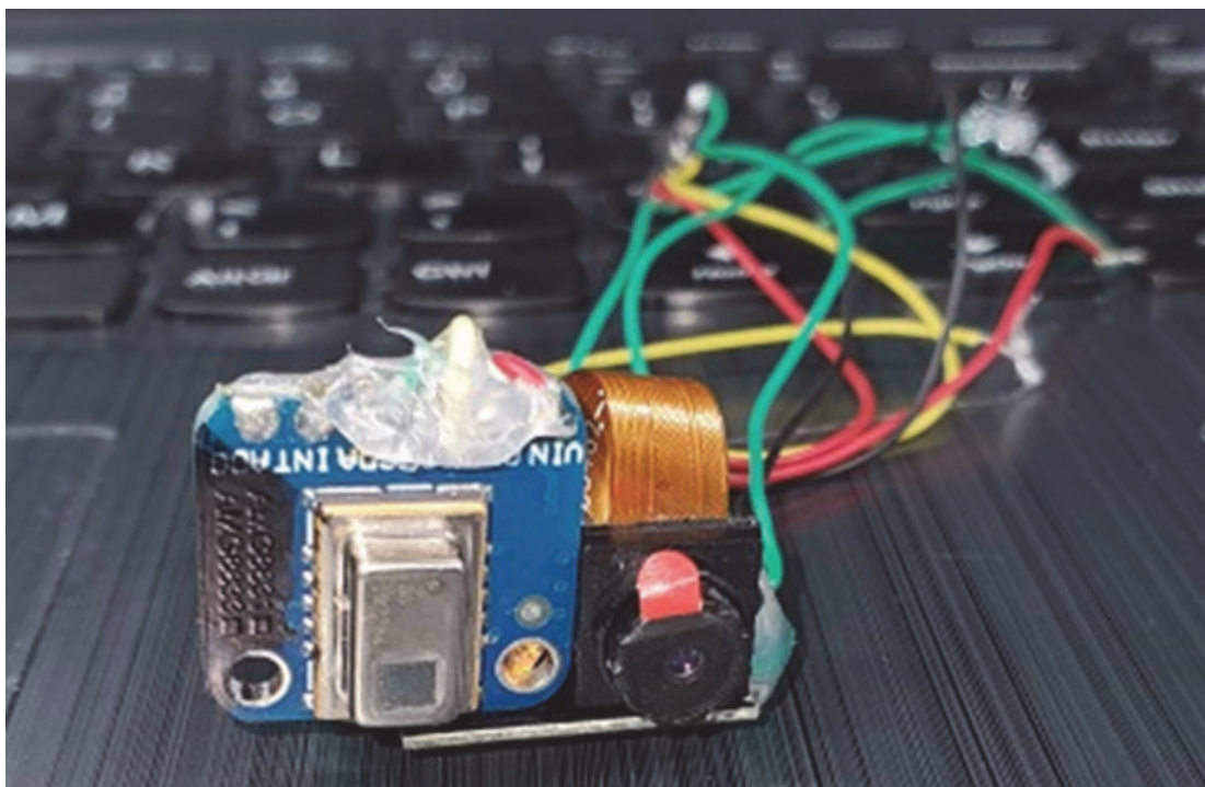
Figure 13: AMG8833 thermal I2C camera with visible wavelength camera in the insect backpack.
