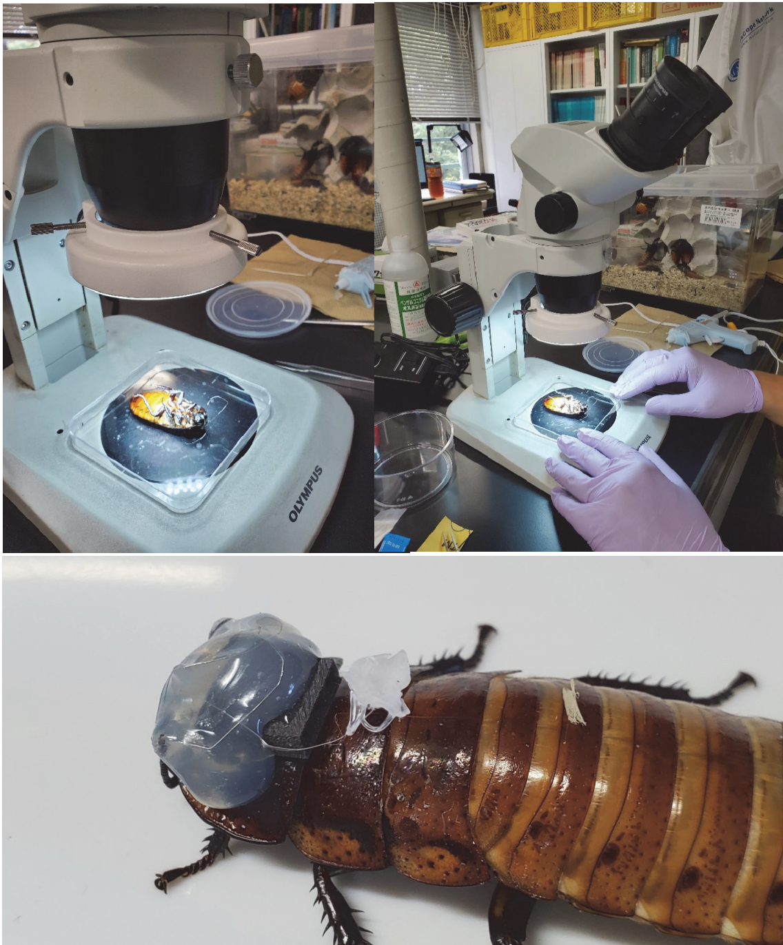
Figure 8: The cockroach was put on the test table below a microscope and the electrodes were inserted through look at the microscope. Surgery done by collaborating researcher Takeshi Suzuki.
