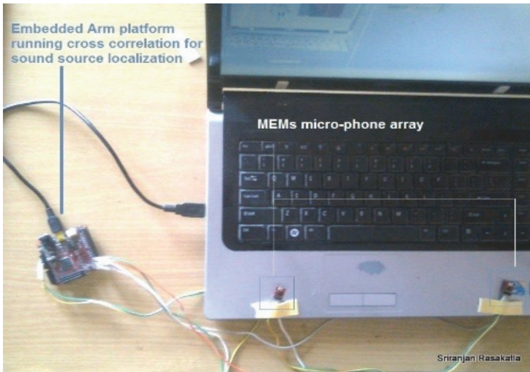
Figure 2: shows MEMs microphone array with sound source localizing done on an ARM microcontroller connected to the laptop via a USB-RS232 serial cable.
