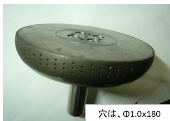
Fig. 2.4 Blade curved surface grinding wheel model
