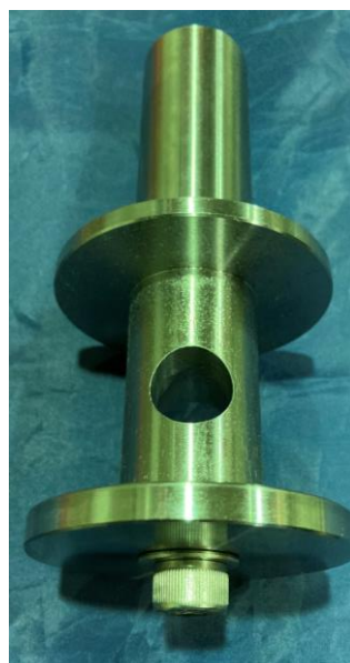
Fig. 5.43 Mounting tool for vitrified grinding wheel
