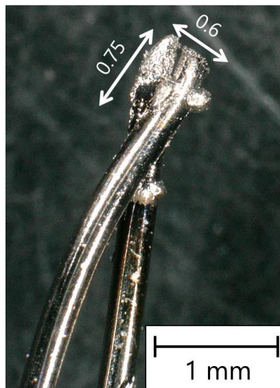
Fig. 5.26 Temperature sensitive point of thermocouple
