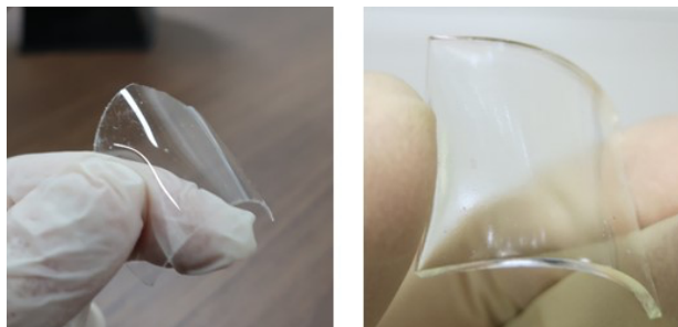
Figure 4.1 Photographic images of UV-curable CNSL-derived polymer films prepared with DMPA photo-initiator (left: 75 \mu\text{m} , right: 750 \mu\text{m} )
