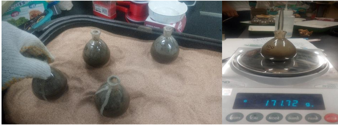
Figure 4. 7: Determination of soil particle density of the paddy soil at Lab soil physics, TUAT, Japan.
