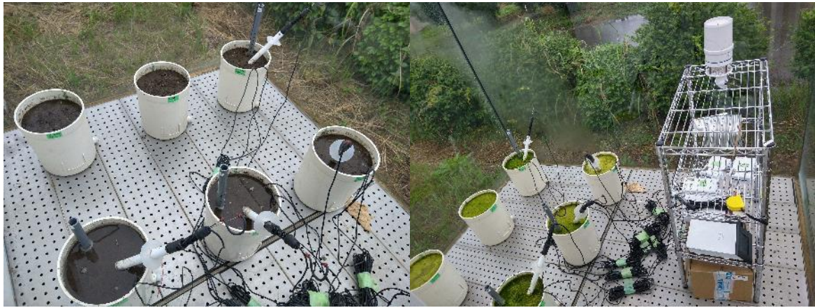
i. Pot experiment set in glass greenhouse (phytotron) with sensors.
