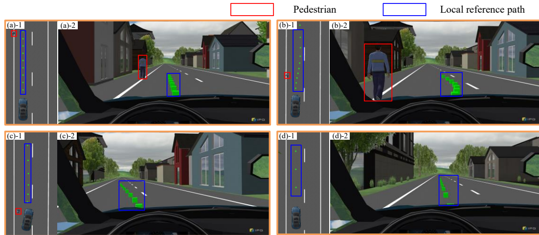
Figure 4.6 Bird's eye view and driver's eye view of T3R HIL test for SFM-based pedestrian avoidance assistance system((*)-1 denotes bird's eye view and (*)-2 denotes driver's eye view): (a) Vehicle approaches pedestrian while cruising; (b) Driver avoids the crossing-road pedestrian according to local reference path; (c) Driver returns to global reference path after avoidance; (d) CA process is over and the vehicle returns to cruising state
