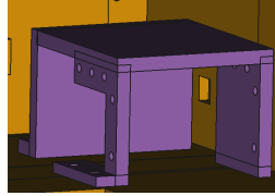
Fig. 8.5: Social Plantroid 's Left servomotor holder.
