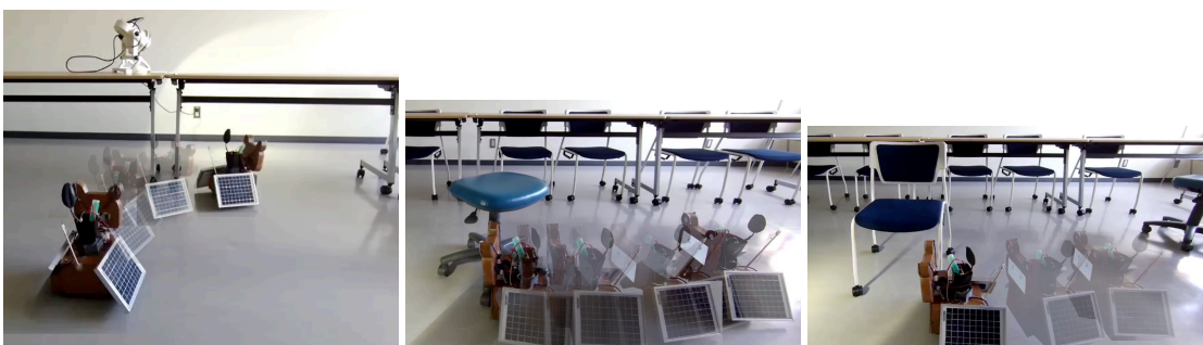
Fig. 8.21: Problematic results, many tries were necessary until Plantroid could avoid the legs of the table (left), could not dodge the chairs after losing sight of its legs (center and right).
