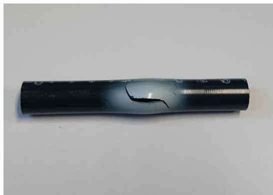
Fig. A.17 Specimen after hydraulic load
