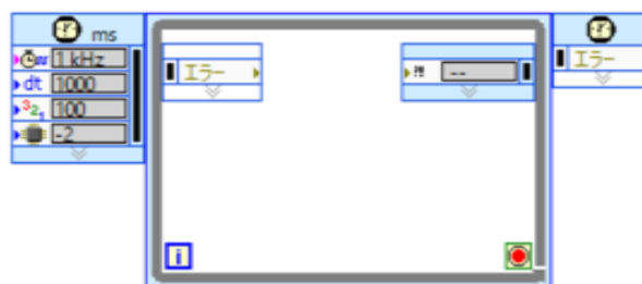
Fig. C.11 Geometry of timing loop function in LabVIEW
