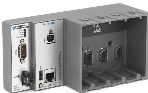
Fig. 2.31 C Series chassis that can be used in Lab VIEW (CompactRIO-NI9063)
