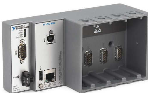
Fig. C.2 C Series chassis that can be used in Lab VIEW (CompactRIO-NI9063)
