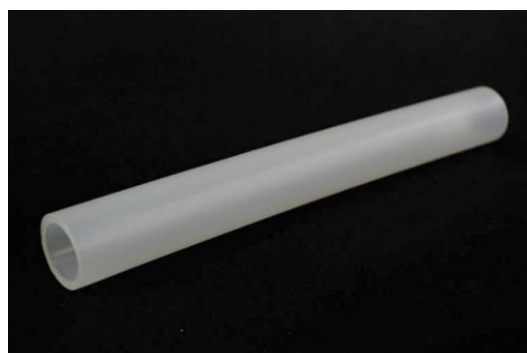
Fig. 3.3 Photograph of circular tube test piece of extruded polyethylene tube
