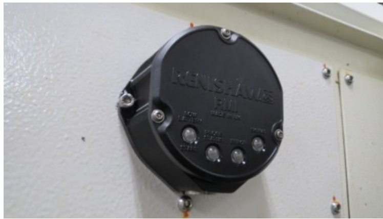
Figure 5.3 Radio machine interface (RMI) of the touch-trigger probe RMP600
