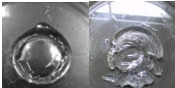
Figure 4-1 PIL gels prepared with 1 mol % of C_{14}M (right) and 3 mol % of C_{14}M (left).
