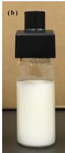
Fig. 2-1. (a) Turbiscan tower (Formulation, Toulouse, France) (b) Turbiscan measuring vial (27mm outside diameter)
