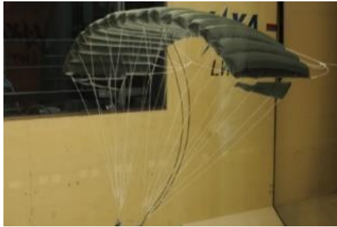
Fig. 2-2 Closed type parafoil (a) Appearance of closed type parafoil (b) Inflation mechanism of closed type parafoil
