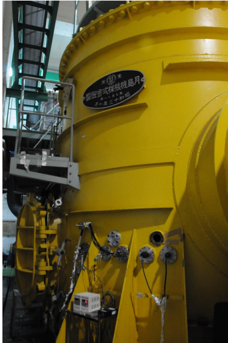
Fig. C-5 Side view of planetary environment wind tunnel.
