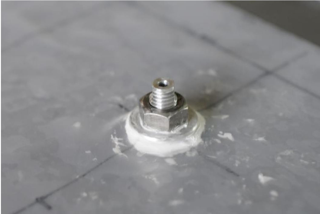
Fig. B-6 Extended picture of gas port.
