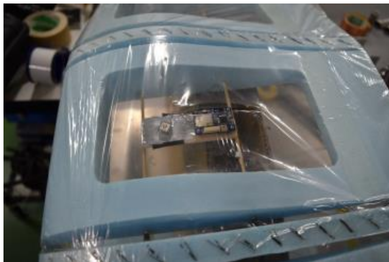
Fig. 4-17 picture of gyro sensor located in the center of the parafoil
