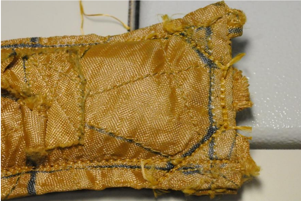
Fig. B-10 Picture of end of strength layer.
