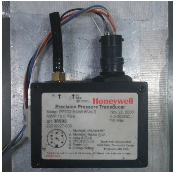
Fig. C-10 Absolute manometer for measurement wind tunnel pressure.
