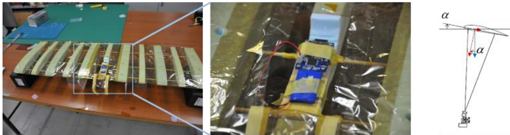
Fig. 3-9 Installation position of a three-axis acceleration sensor-logger (a) Appearance of the installation position of the sensor-logger (b) Definition of acquired acceleration and gravitational acceleration used in the calculation of the angle of attack of test model
