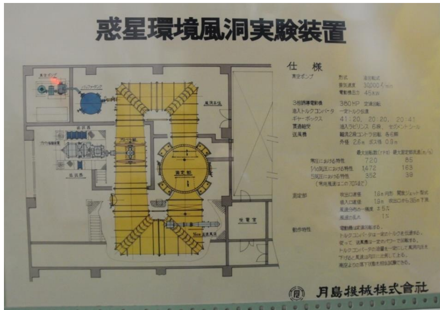
Fig. C-4 Specification of planetary environment wind tunnel.
