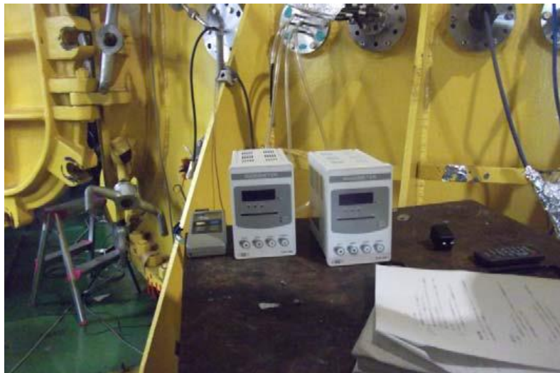
Fig. C-11 Differential manometer for measurement pitot pressure.
