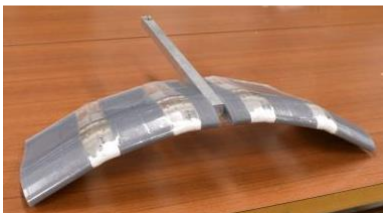
Fig. C-3 Picture of arc anhedral wing model for wind tunnel test.
