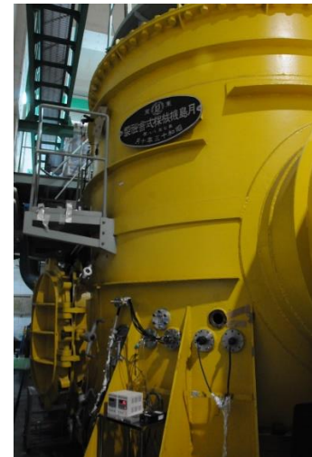
Fig. 2-9 Planetary environment wind tunnel. (a) specification of planetary environment wind tunnel (b) Outside view the wind tunnel
