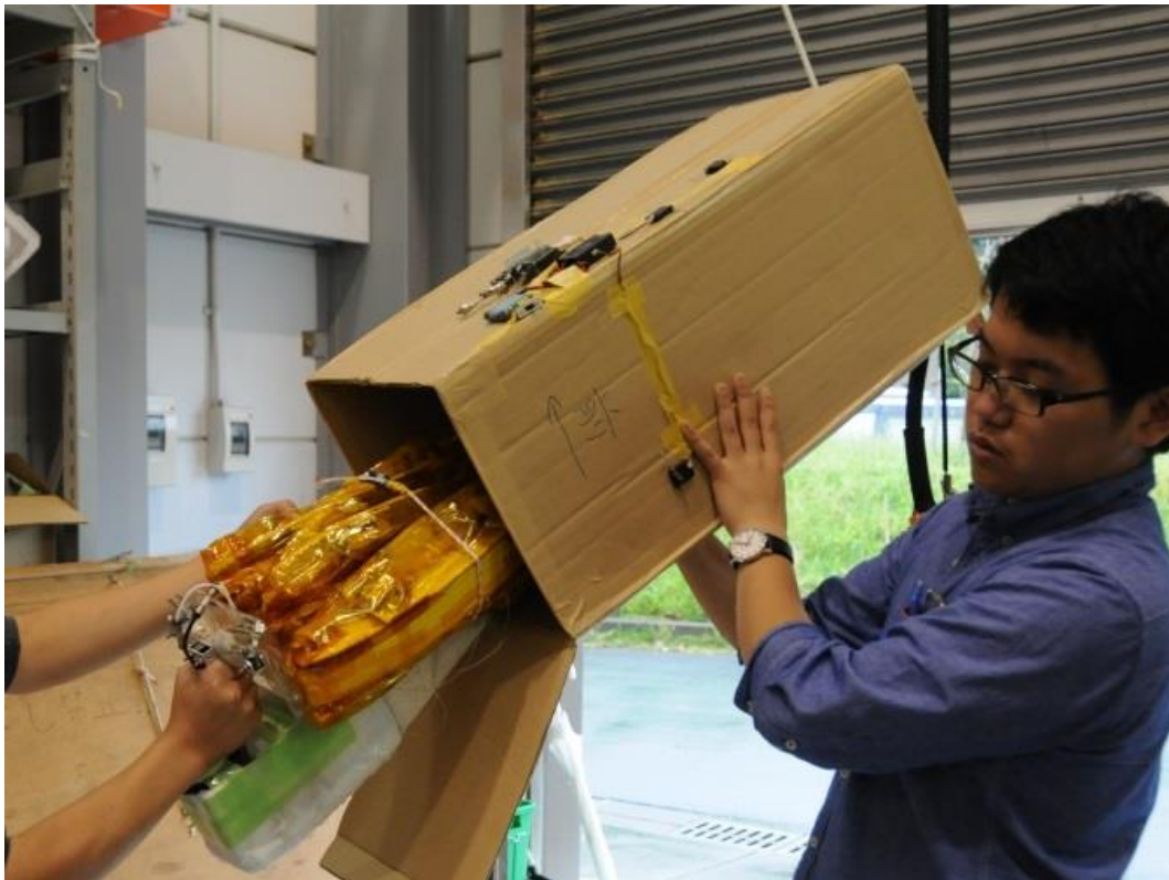
Fig. 2-32 Release system for helicopter drop test
