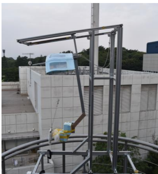
Fig. 4-19 Parafoil loaded in injection device
