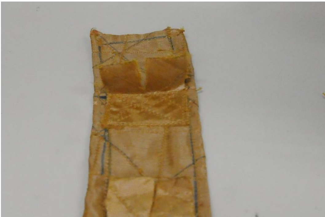
Fig. B-5 picture of tab to fix the rib.
