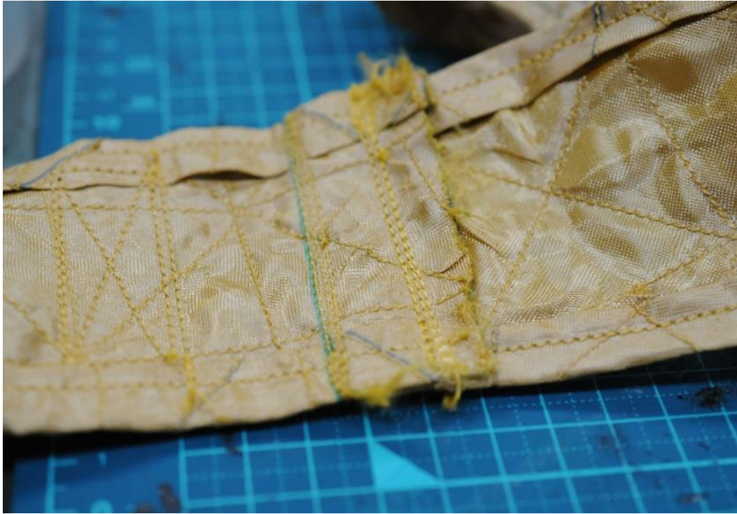
Fig. B-4 Extended picture of connect part of strength layer.
