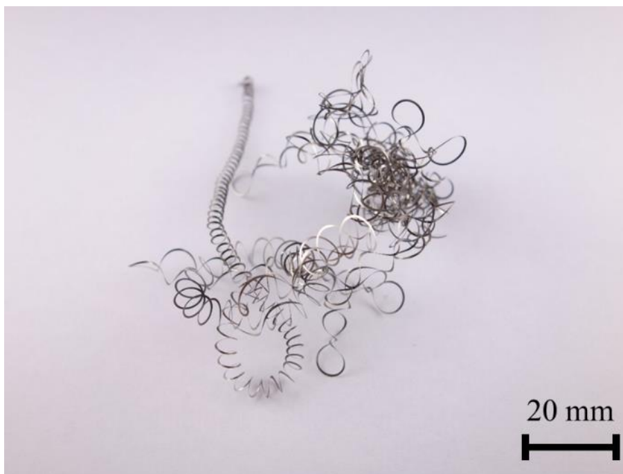
(a) Conventional cutting, S = 3752 \text{ min}^{-1}
