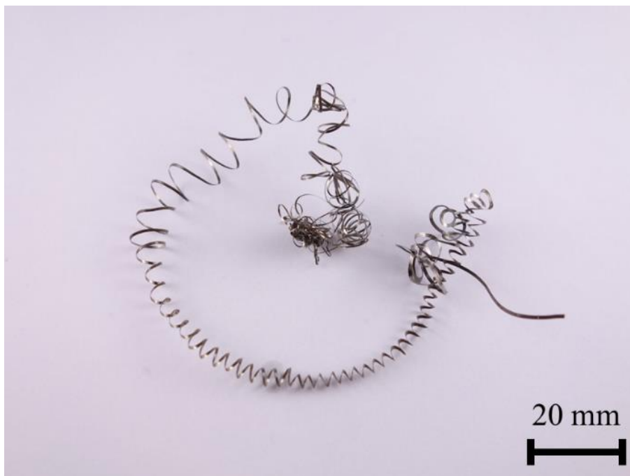
(a) Conventional cutting, S = 3752 \text{ min}^{-1}
