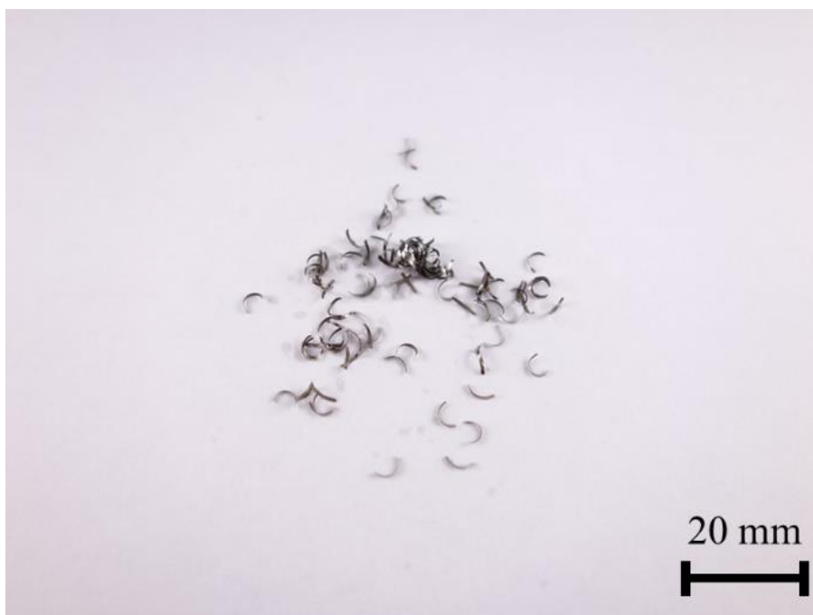
(b) LFV, Q = 2.0 , D = 1.5 , f_v = 93.8 \text{ Hz} , S = 3752 \text{ min}^{-1}
