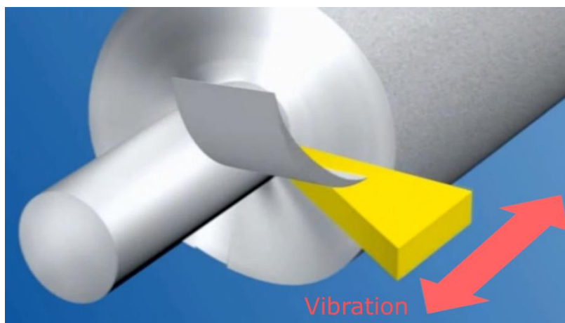
Fig. 2.4 Direction of LFV vibration in turning process.
