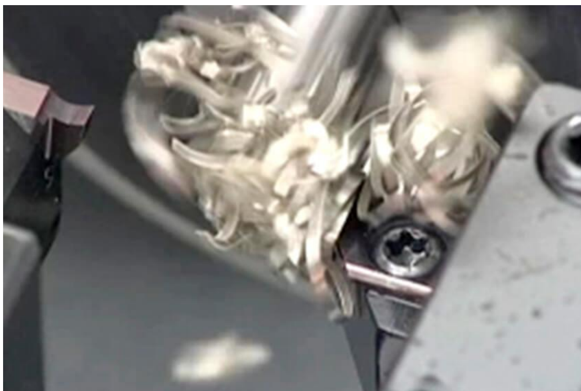
Fig. 1.1 Chip entanglement in turning process[5].
