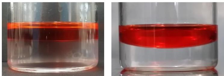
Fig. 5-1 Photo images of samples with EPDME (left) and without EPDME (right). Oil amount is 2.8 g. Oil was dyed by Sudan III.
