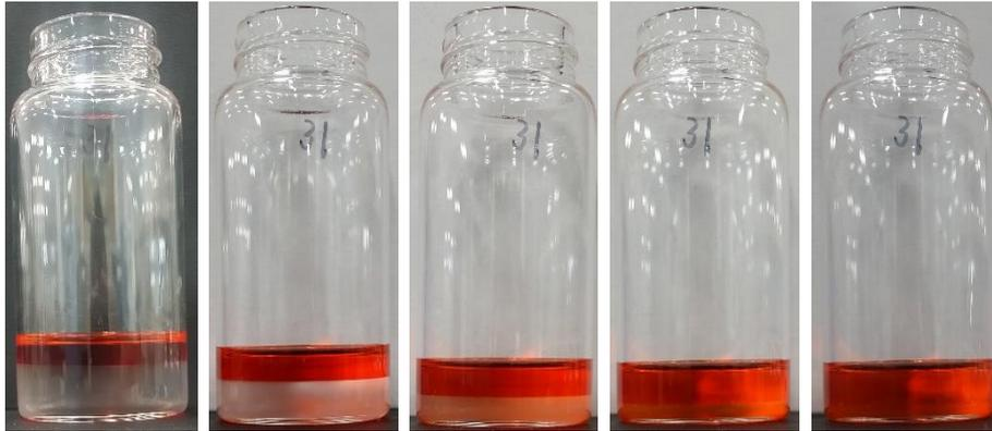
Fig. 5-3 Images of EPDME (9/2) sample during drying. The oil amount was 2.8 g. Images were taken at 0 min, 5475 min, 8946 min, 12875 min and 14697 min from left to right. The height of vessel is 73.5 mm.
