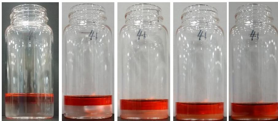
Fig. 5-5 Images of EPDME (14/7) sample during drying. The amount of oil was 2.8 g. Images were taken at 0 min, 5475 min, 8946 min, 12875 min and 16994 min from left to right. The height of vessel is 73.5 mm
