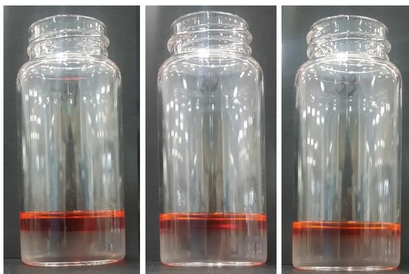
Fig. 5-2 Photo images of the initial samples before drying. The amount of oil is 2.8 g, 2.0 g and 1.4 g from left to right, respectively. The oil phase was dyed by Sudan III.
