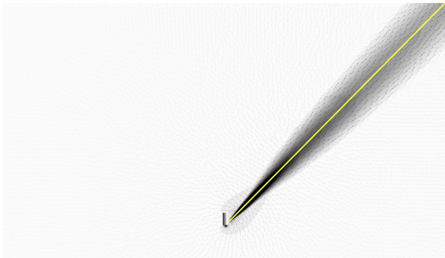
Fig. 2.11 Result of simulation for a jet discharged 45^\circ backward to one side. The yellow line shows the initial jet discharge direction.
