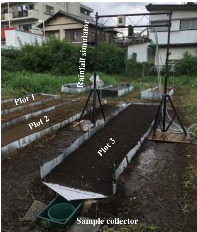
Figure 5.1. The upland bare soil pollutant runoff experiment in Sakaecho, Tokyo (2017) (Yadav and Watanabe, 2018)
