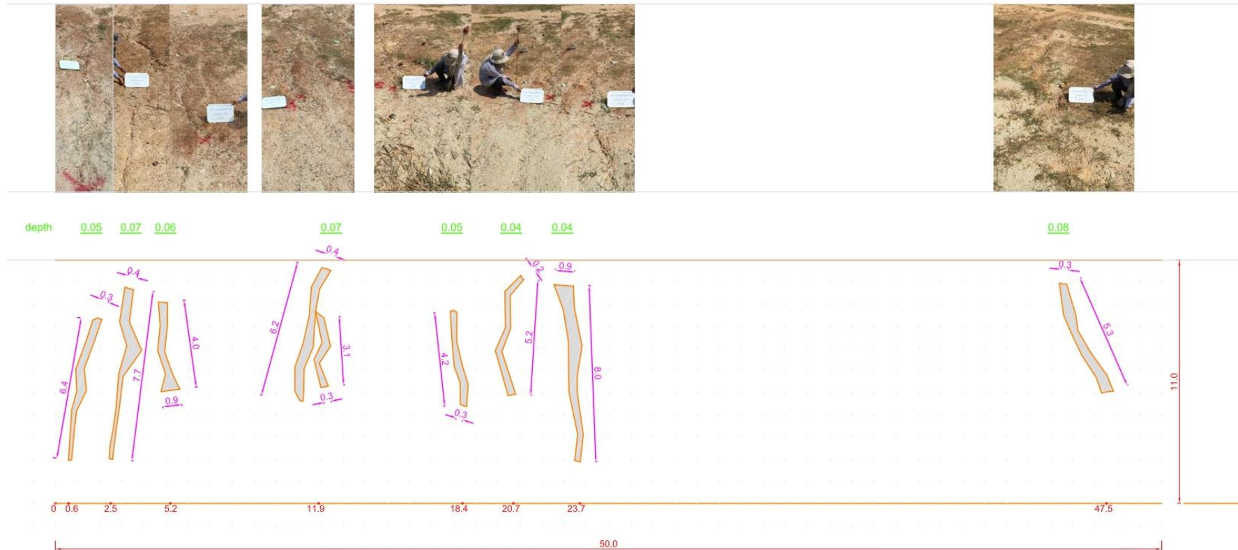
Fig 3. 5 The schematic diagram of erosion measurement in Thomney site, Takeo province, Cambodia
