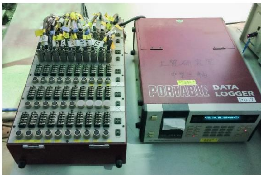
Fig 4. 10 Data logger and switcher to record the pore water pressure (Chueasamat, 2018)
