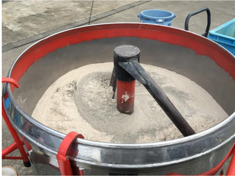
Fig 6. 5 Electric mixer uses to mix soil cement
