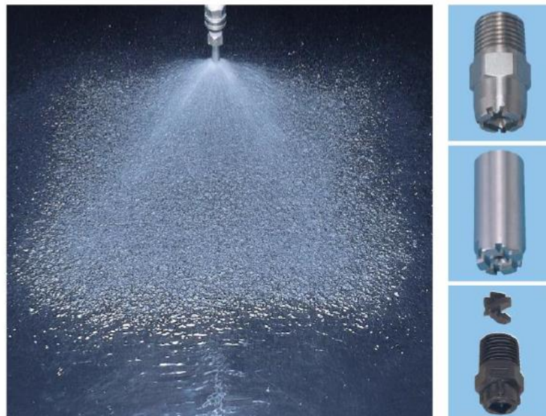
Fig 4. 7 Spray nozzle used in soil slope model erosion resistance test (Chueasamat, 2018)
