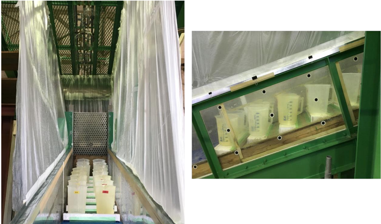
Fig 6. 1 Rainfall Calibration process by using measuring cups to capture the rainwater at the specific duration
