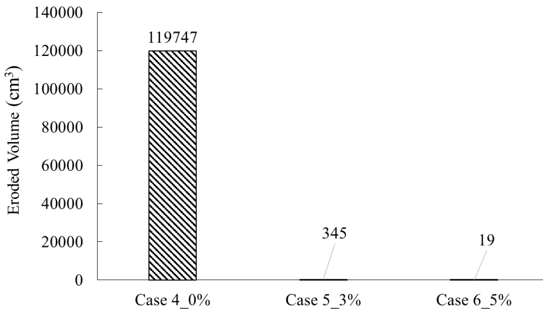
Fig 6. 15 The estimated surface eroded volume under 100 mm h -1
