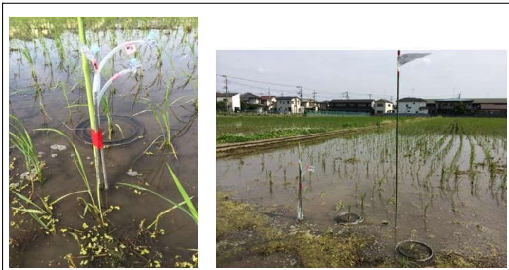
Figure 13 Site setup the soil gas sampling tube buried in the paddy field in duplicated at the six CC method sampling points
