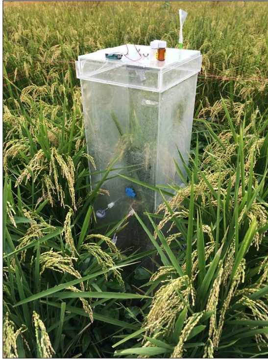
Figure 7 Transparent closed chamber cover rice for gases sampling on rice paddy field at 90 DAT
