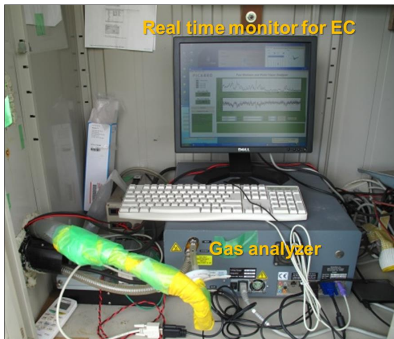
Figure 10 The closed-path eddy covariance system, the \text{CH}_4/\text{H}_2\text{O} closed-path gas analyzer and the real time monitor located inside an instrument box at 5 m far from EC tower
