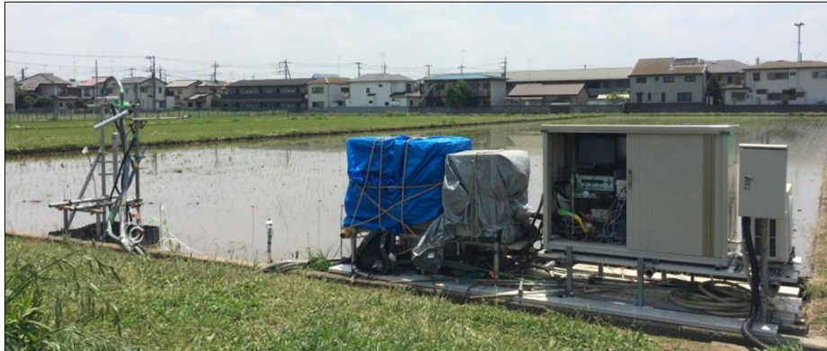
Figure 9 Eddy Covariance system set up with eddy covariance tower and an instruments box at 5 m far from the EC tower
