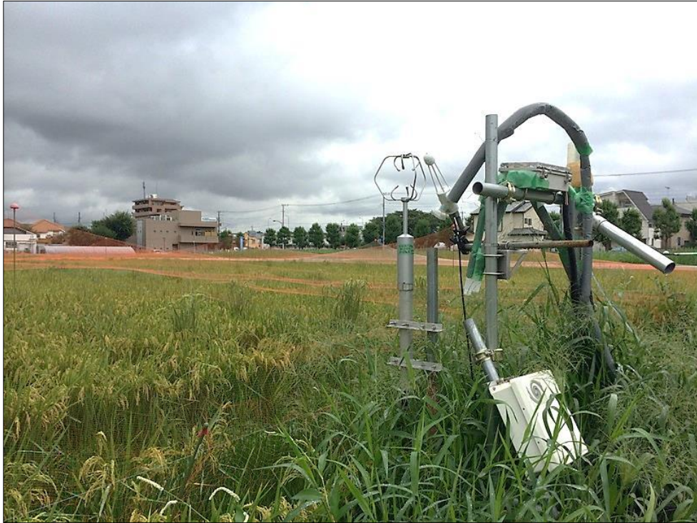
Figure 8 Eddy Covariance set up consisted with open-path CO 2 /H 2 O gas analyzer and closed-path CH 4 /H 2 O sampling tube set up with a three dimensional sonic anemometer
