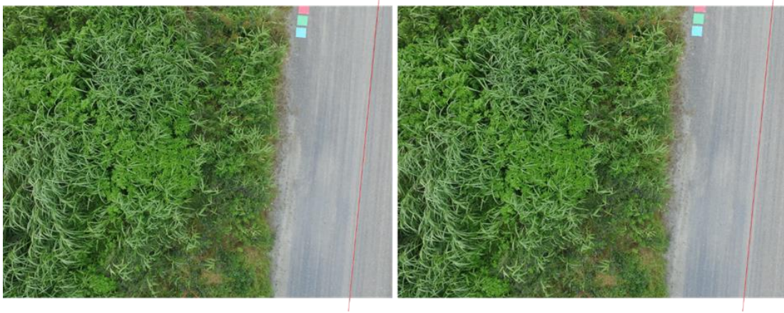
Figure 3-8 Original image (left) and undistorted image (right).
