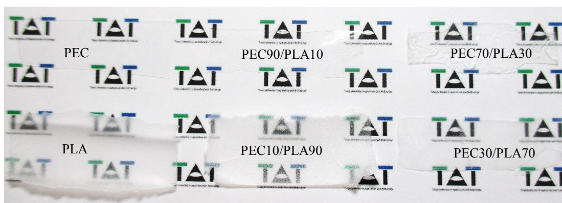
Fig. 2-5 Images of PEC/PLA blends (as cast).
