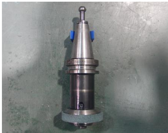
Fig. 2.8 Developed device utilizing through-spindle system
