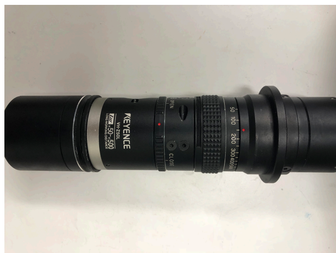
Fig. 2.8 Lens with long working distance
