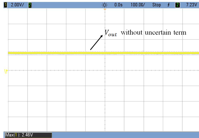
Figure 3.11: Output voltage of the WPT system with the certain distance.
