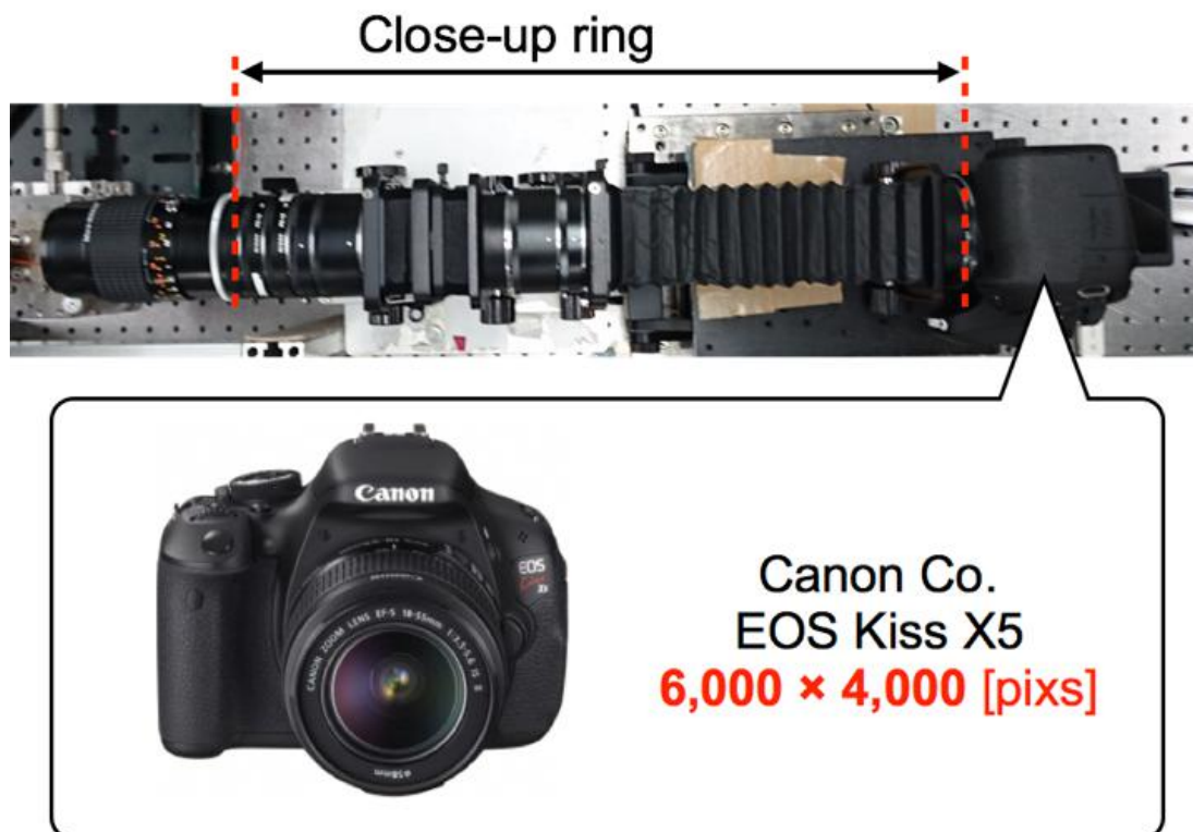
Fig. 4.2 Setup of camera for high-resolution photography
