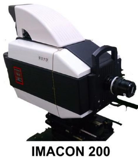
Fig. 2.8 IMACON 200 (ultra high-speed video camera) for observation of plasmas.
