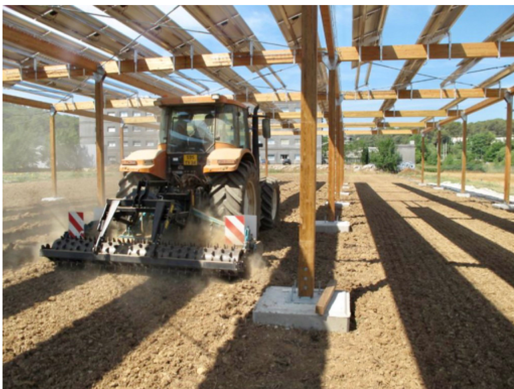
図 4-9 モンペラ大学（仏）の Agrivoltaic 実験設備の様子 Source: C. Dupraz, “From Agroforestry to Agrivoltaism :scientific evidence for the unexpectedly high productivity of new dual systems”
