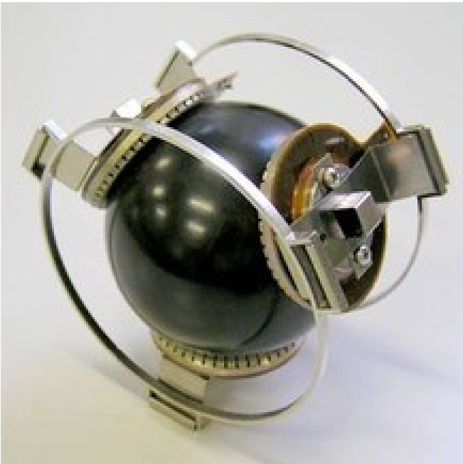
Fig. 1.5 Spherical Ultrasonic Motor with 3 stators
