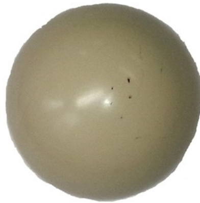
Fig. 8.13 Damage occurred on the surface of spherical rotor
