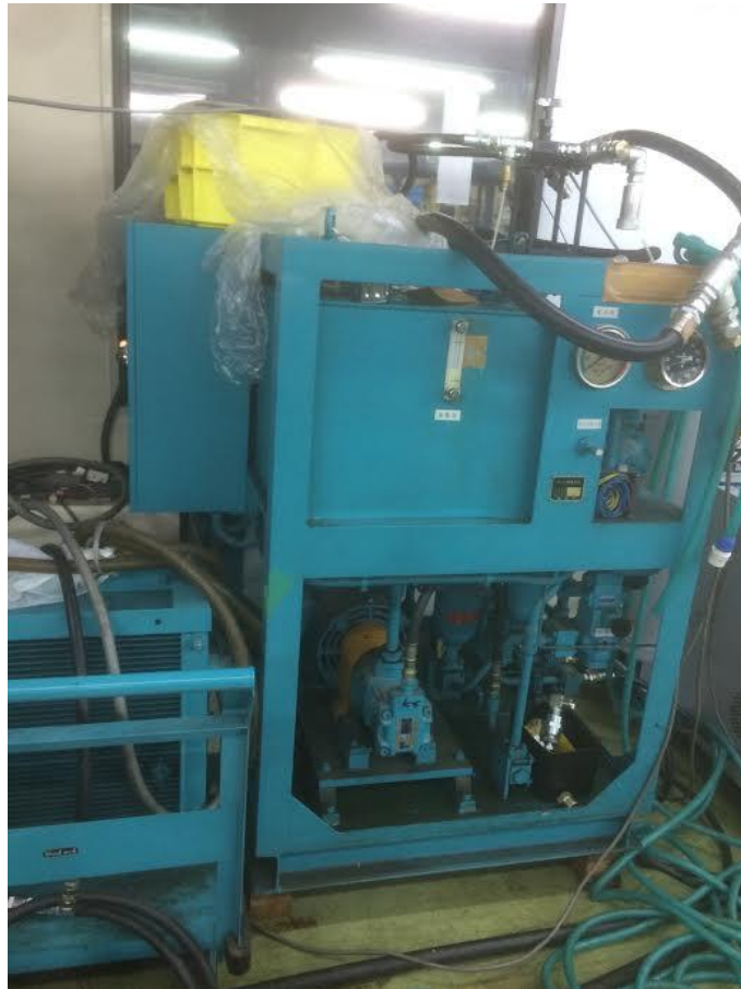
Fig. 6.7 Hydraulic power unit 5.5 kW
