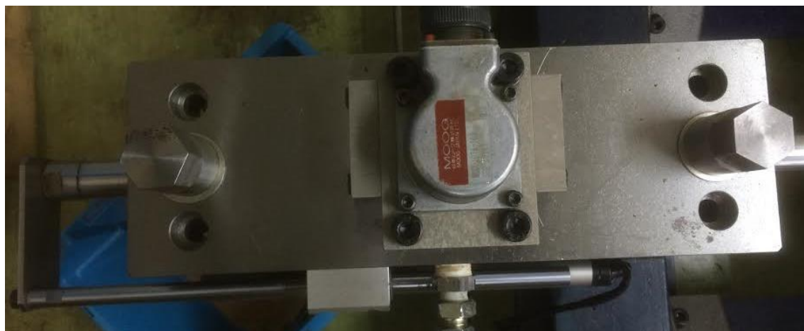
Fig. 6.6 Oil hydraulic cylinder (FF-WE-1LA32AN150AOD)
