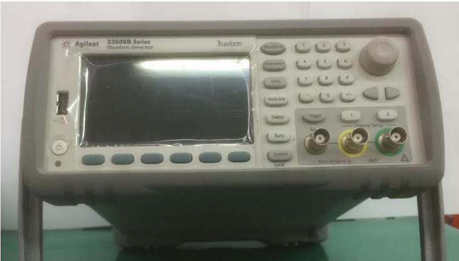
Fig. 6.3 Multi-function generator (33512B) Table 6.3 Specification of Multi-function generator (33512B)
