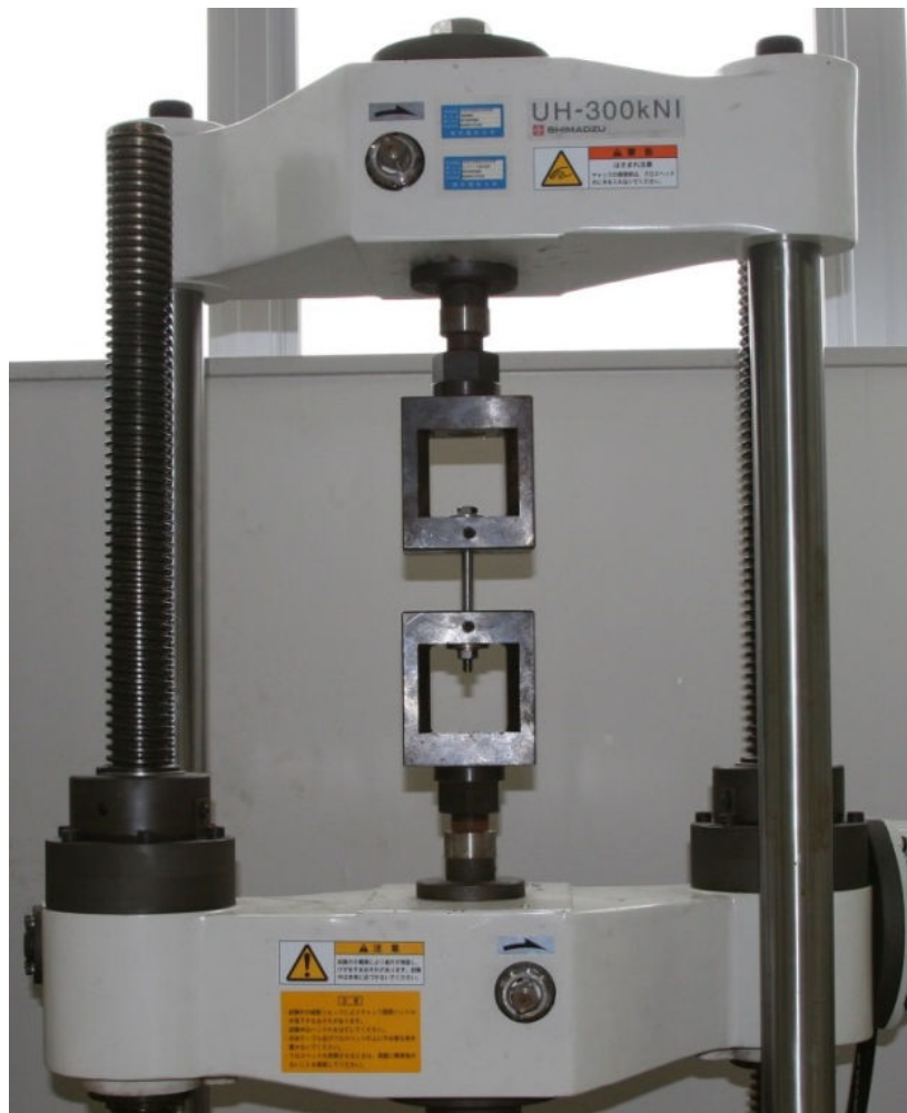
Fig. 3.9 Experimental apparatus of tensile strength tests
