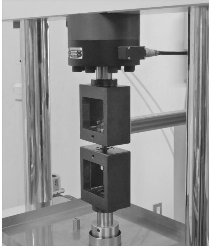
(a) Test rig installed in the hydraulic servo-controlled fatigue test machine
