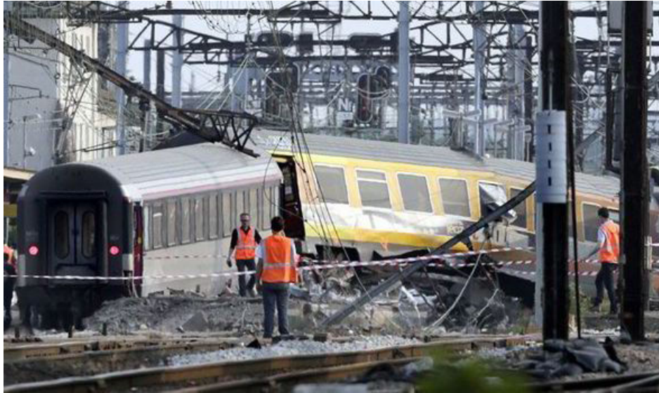
Fig. 1.8 Paris rail crash by loose bolt 22)
