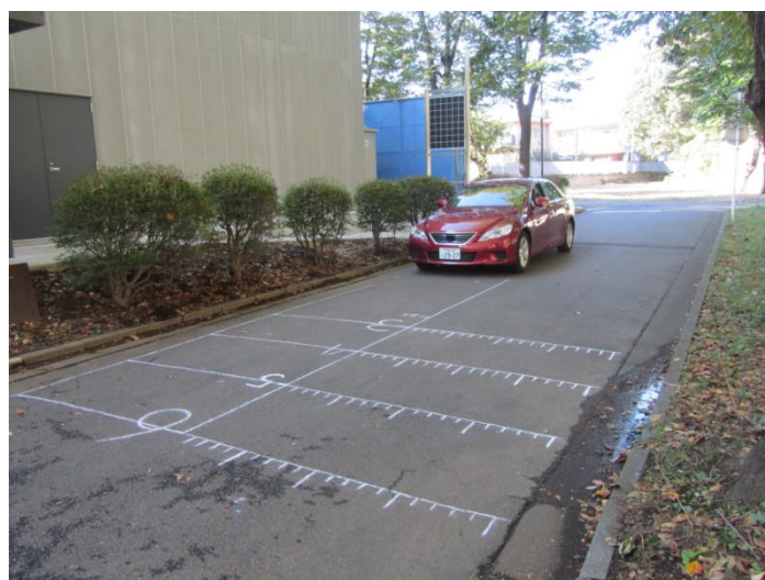
Fig. 2.1.8 Preparation for Measurement of lateral distance from vehicle
