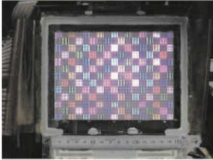
Figure 2.9 Emission image of fabricated 7.6-in.-diagonal prototype model [63].
