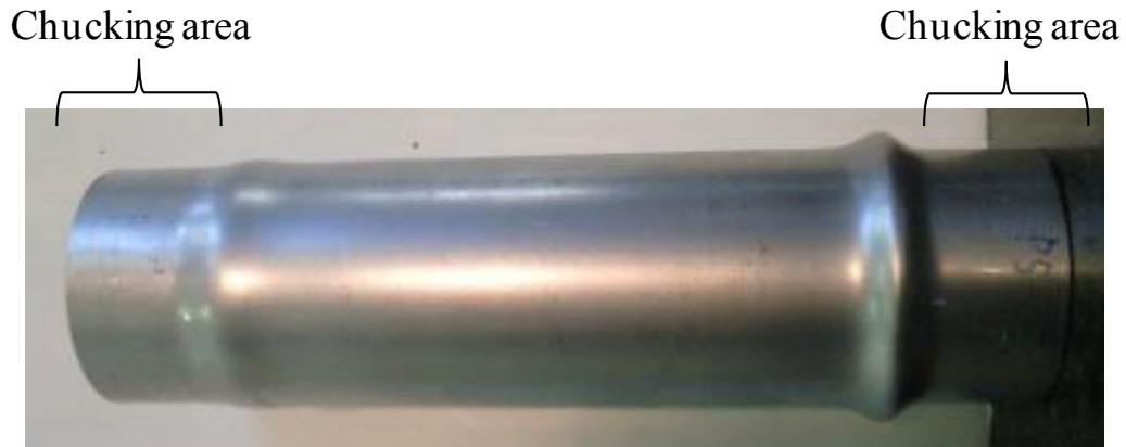
Fig. 6-7 The specimen after the axial compression test under constant internal pressure.
