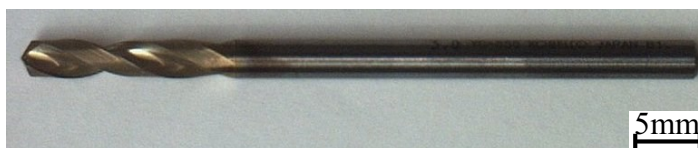
Fig. 2-8 Photograph of TiAlN coated cemented carbide drill
