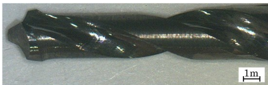
Fig. 3-10 Photograph of ground drill
