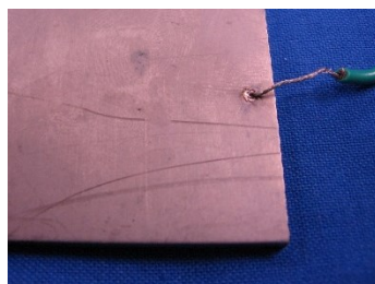
Fig. 3-3 Photograph of copper wire welding point
