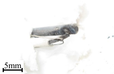
Fig. 3-11 Carbide with welded titanium and thermocouple in electric furnace
