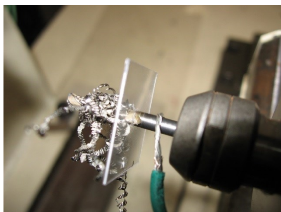
Fig. 3-5 Contact at drill shank and chip stopper
