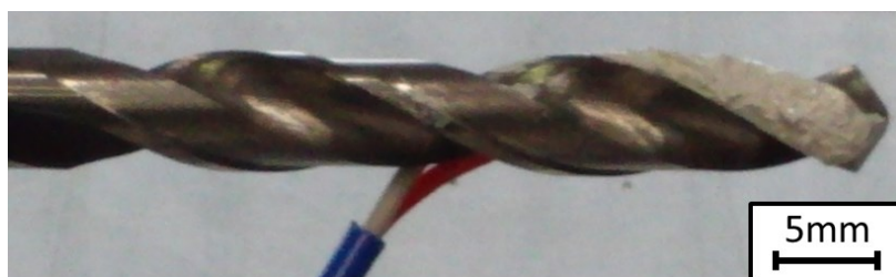
Fig. 4-18 Side view of embedded thermocouple
