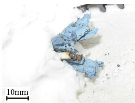
Fig. 3-14 Fragmented carbide after heat
