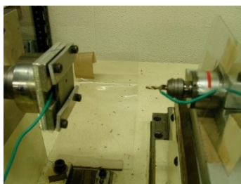
Fig. 3-2 Photograph of tool-work-thermocouple method
