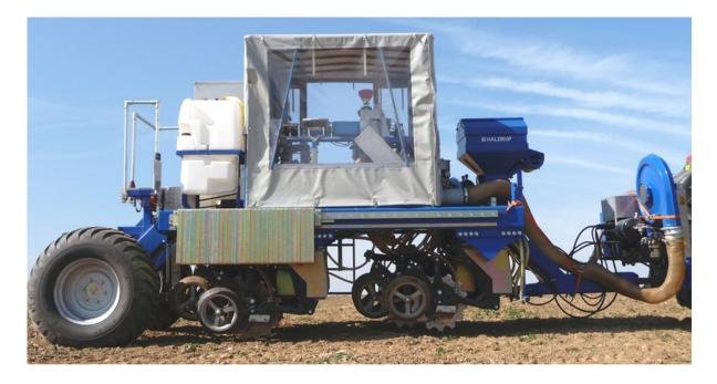
Fig. A 1. Prototype plot seeder with cross-slot openers.
