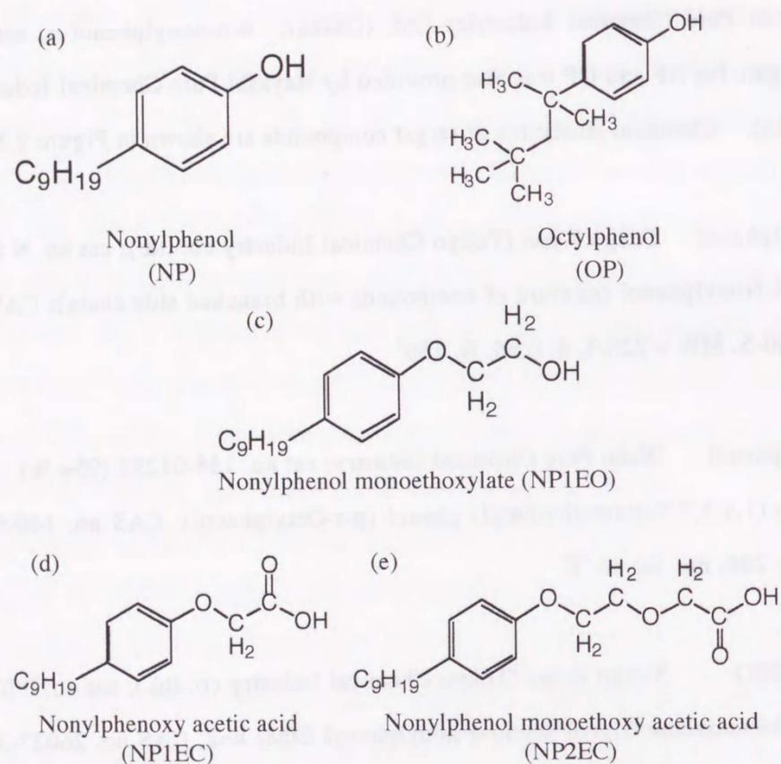
**Figure 2.1** Chemical structures of the target compounds. Nonylphenol (NP, a), octylphenol (OP, b), nonylphenol monoethoxylate (NP1EO, c), nonylphenoxy acetic acid (NP1EC, d), and nonylphenol monoethoxy acetic acid (NP2EC, e). C<sub>9</sub>H<sub>19</sub> is highly branched alkyl chain.
