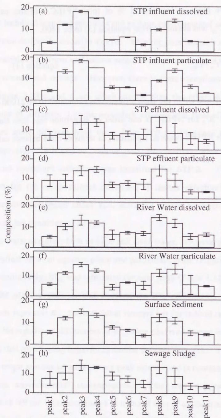
**Figure 3.28** Individual peak composition of NP in the dissolved (a) and particulate (b) phases in the influents (influent and primary effluent), dissolved (c) and particulate (d) phases in the effluents (secondary and final effluent) of STPs, dissolved (e) and particulate (f) phases in the river waters, surface sediments (g), and sewage sludge (h).
