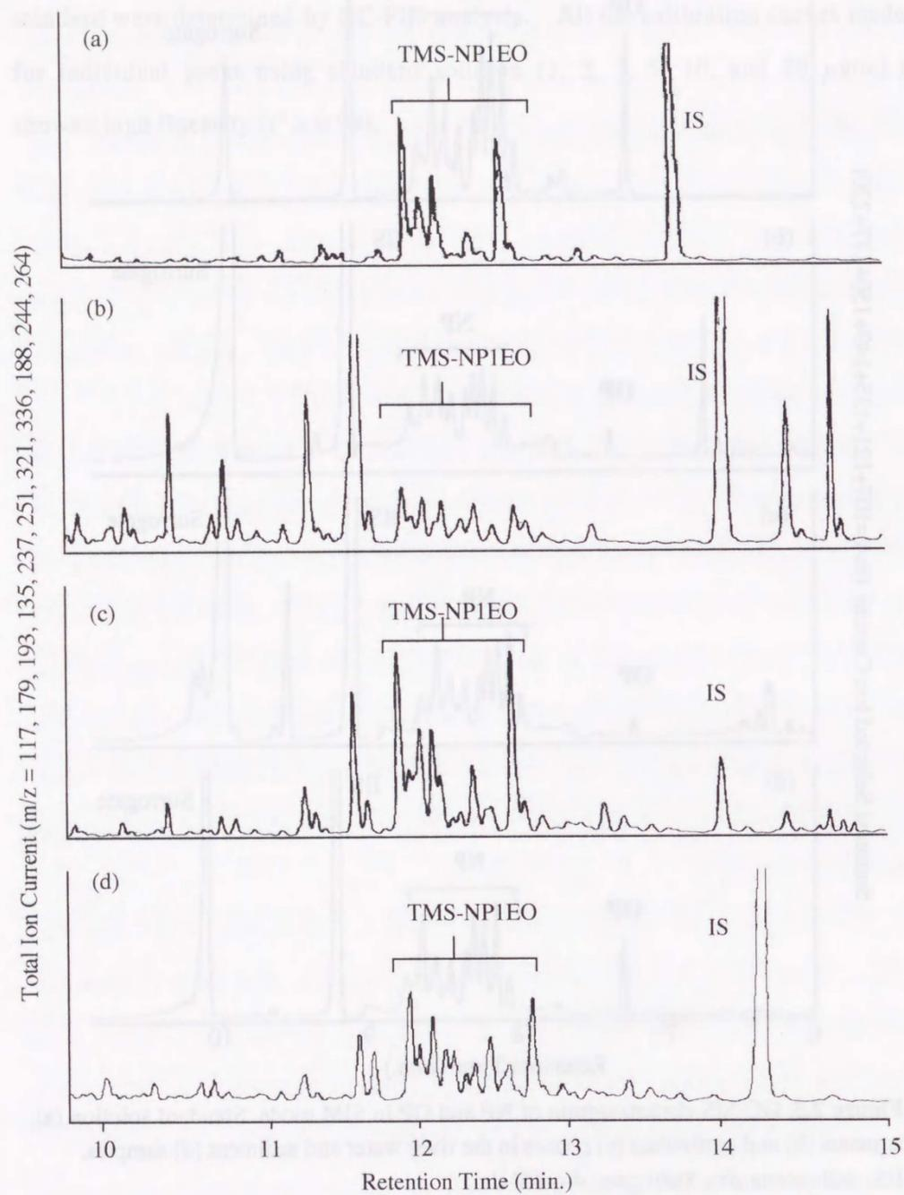
**Figure 2.6** GC-MS chromatogram of trimethylsilylated NP1EO in SIM mode. Standard solution (a), aqueous (b) and particulate (c) phases in the river water and sediment (d). TMS-NP1EO; trimethylsilylated NP1EO, IS; p-terphenyl-*d*14.
