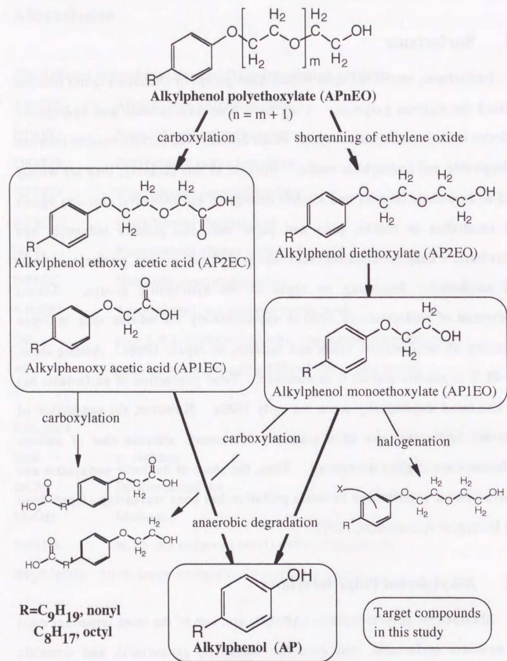
Figure 1.1 Biodegradation pathways of alkylphenol polyethoxylates (APnEO).
