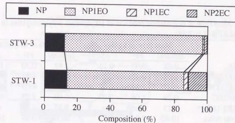
**Figure 3.14** Variation in composition of nonylphenolic compounds in activated sludge collected from STW-3 and STW-1.
