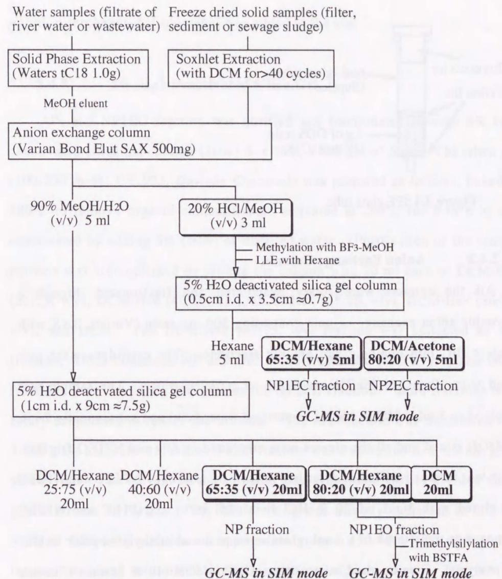
Figure 2.3 The scheme of analytical procedure for NP, OP, NP1EO, NP1EC and NP2EC.
