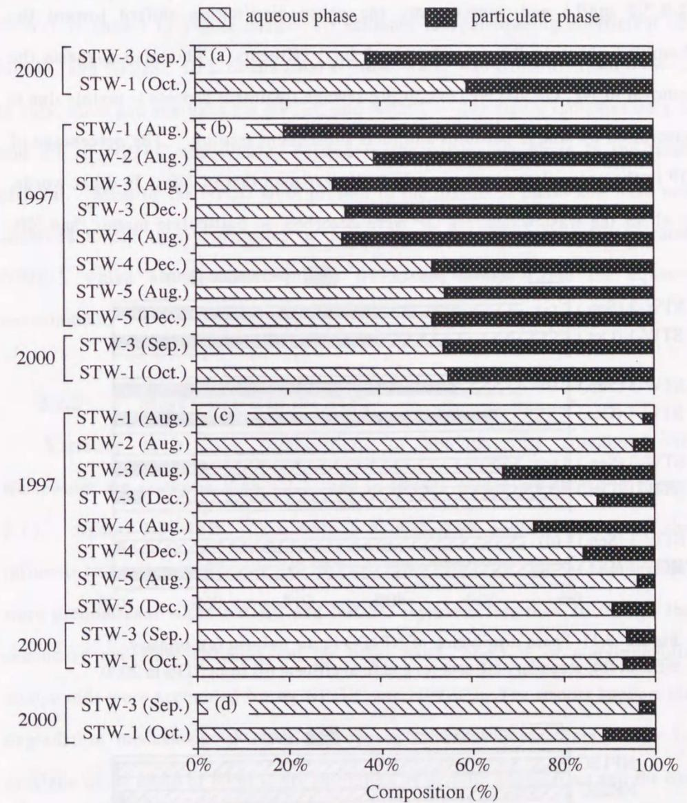
Figure 3.10 Phase distribution of OP in the influent (a), primary effluent (b), secondary effluent (c) and final effluent (d) from STPs.
