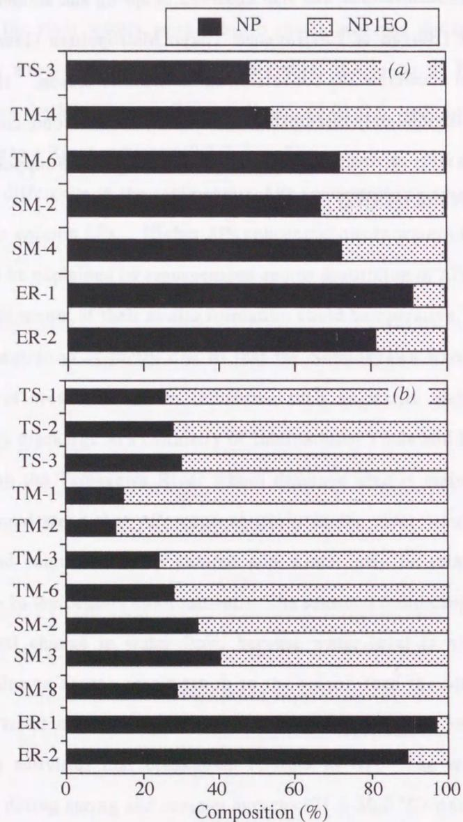
Figure 3.31 Relative composition of NP and NP1EO in the river sediment (a) and river water (b).
