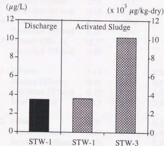
**Figure 3.4** NP1EC concentration in the final effluent and activated sludge (preliminary research).
