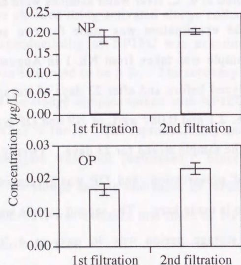
Figure 3.1 APs concentrations in the single- and double-filtered samples.
