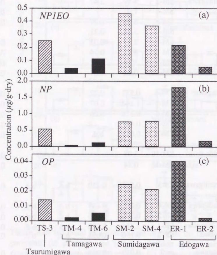
Figure 3.29 Concentrations of NP1EO (a), NP (b), and OP (c) in the river sediments.
