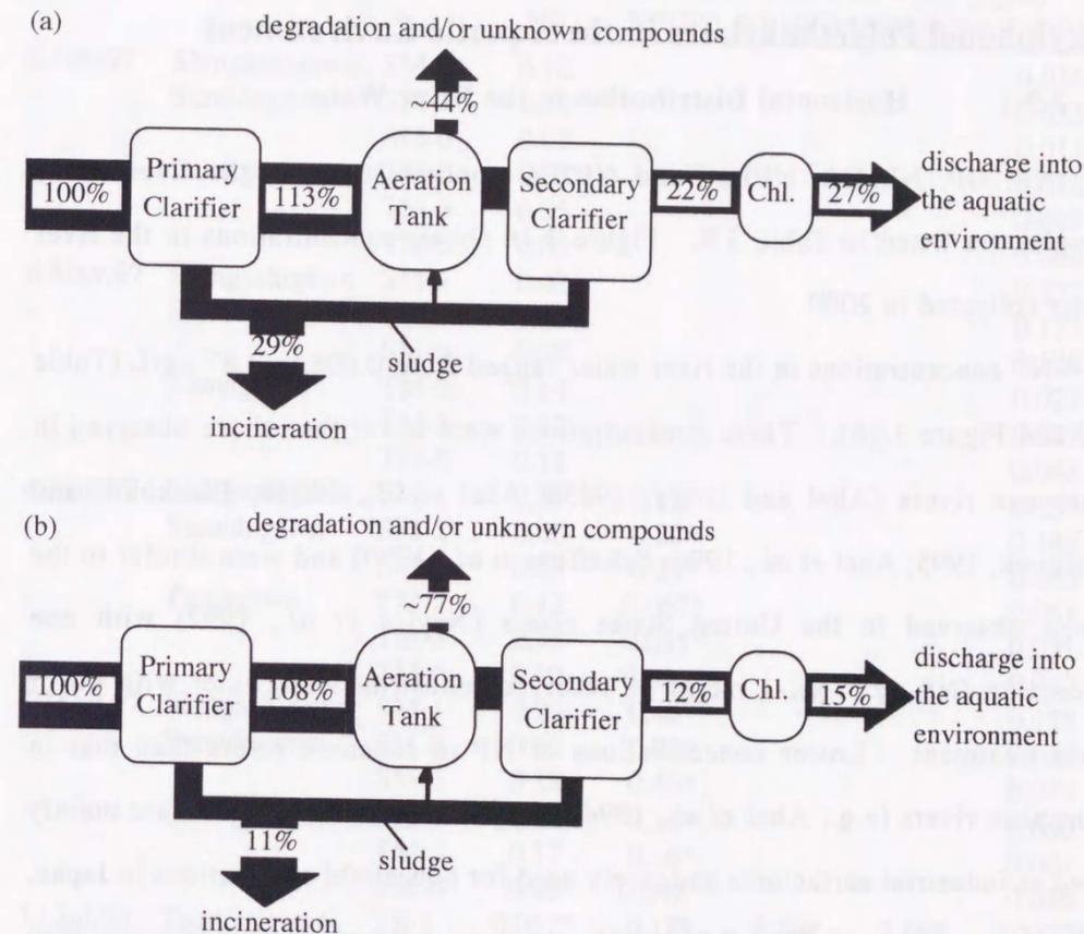
**Figure 3.15** Calculated mass flow of nonylphenolic compounds in STW-3 (a) and STW-1 (b) (molar basis) in 2000. Chl.; chlorination.
