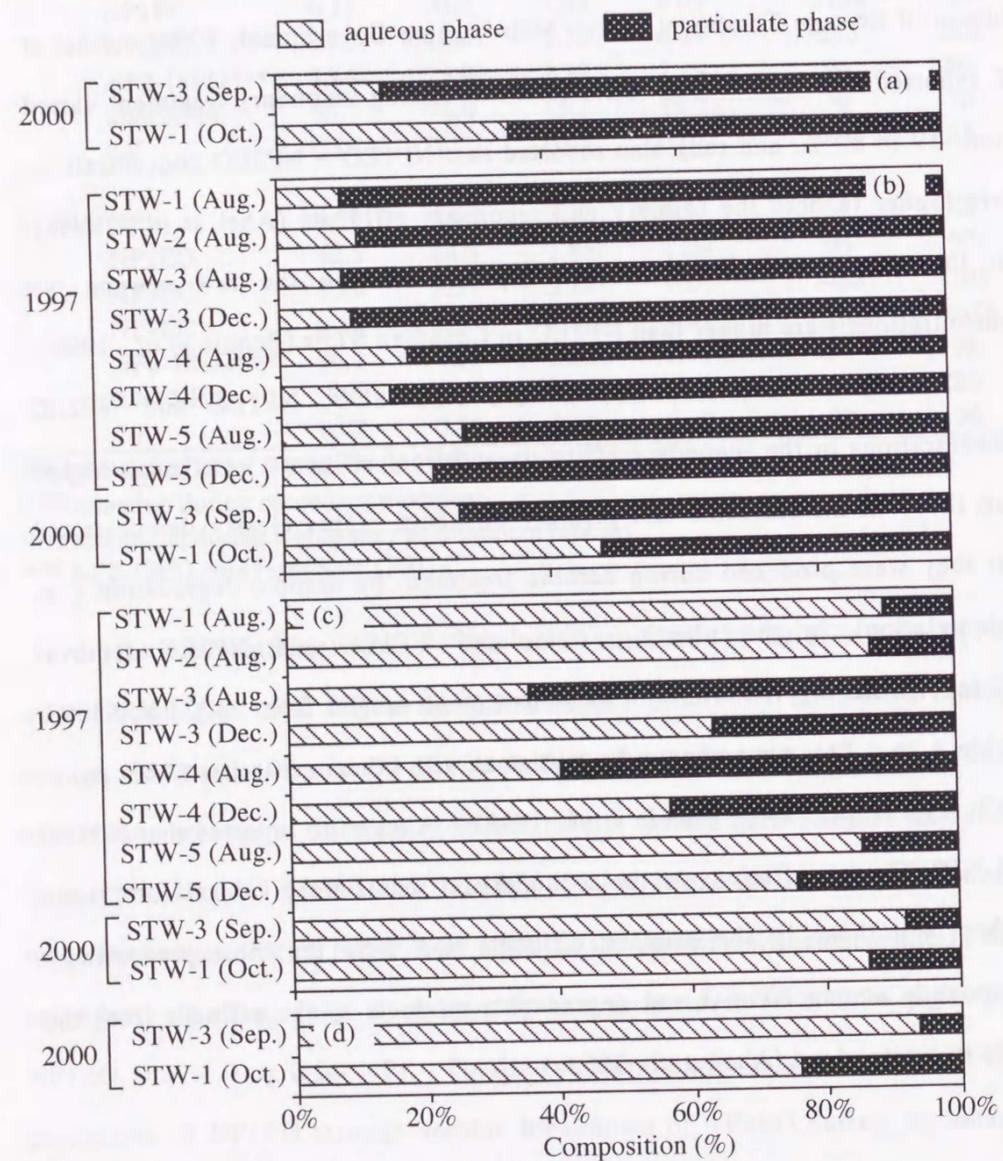
Figure 3.9 Phase distribution of NP in the influent (a), primary effluent (b), secondary effluent (c) and final effluent (d) from STPs.
