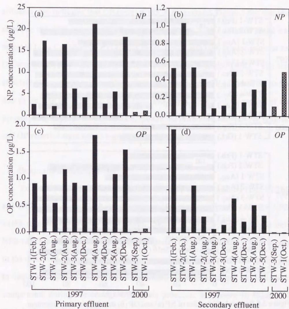
**Figure 3.5** NP (a, b) and OP (c, d) concentrations in the primary (a, c) and secondary (b, d) effluents in the sewage treatment plants.
