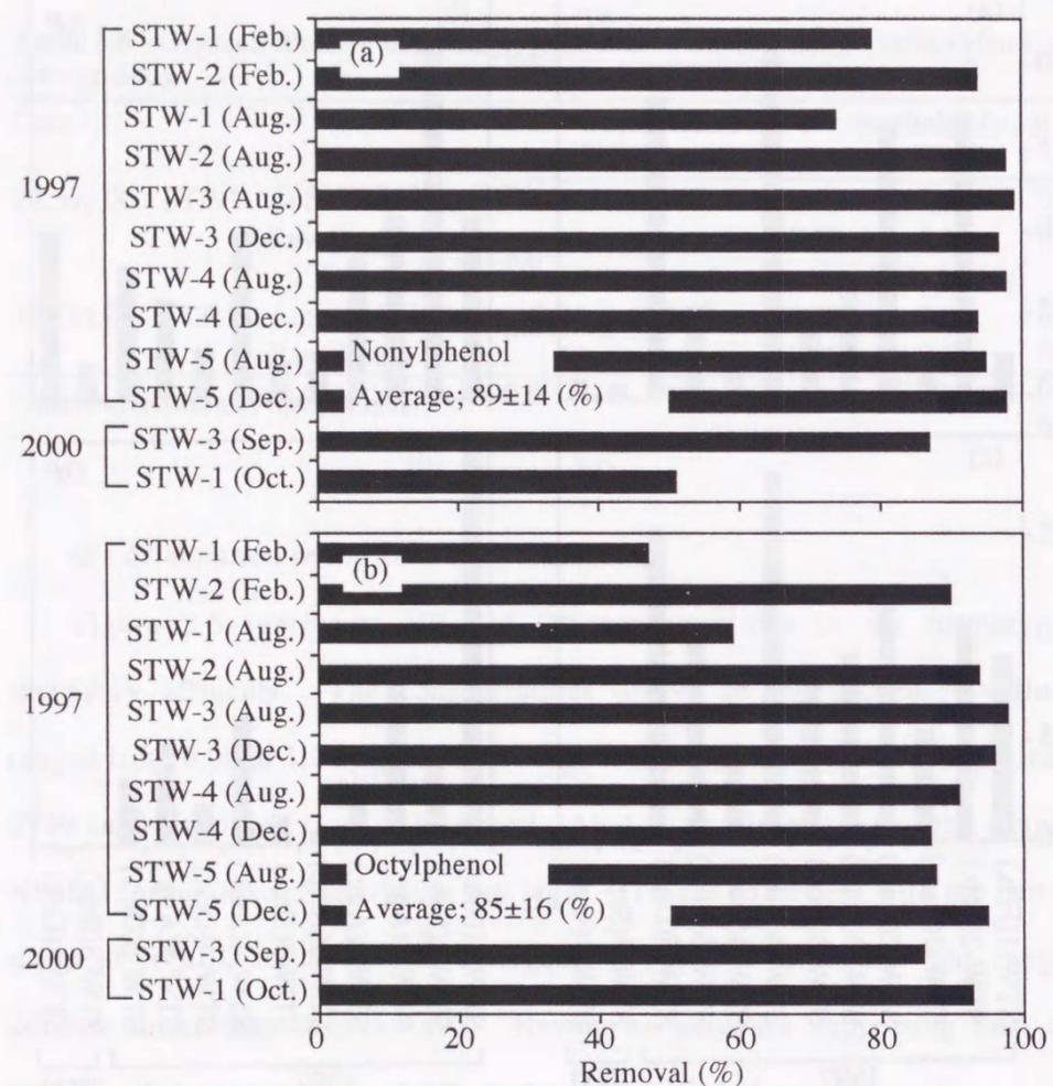
Figure 3.6 Removal efficiencies of NP (a) and OP (b) during secondary treatment.
