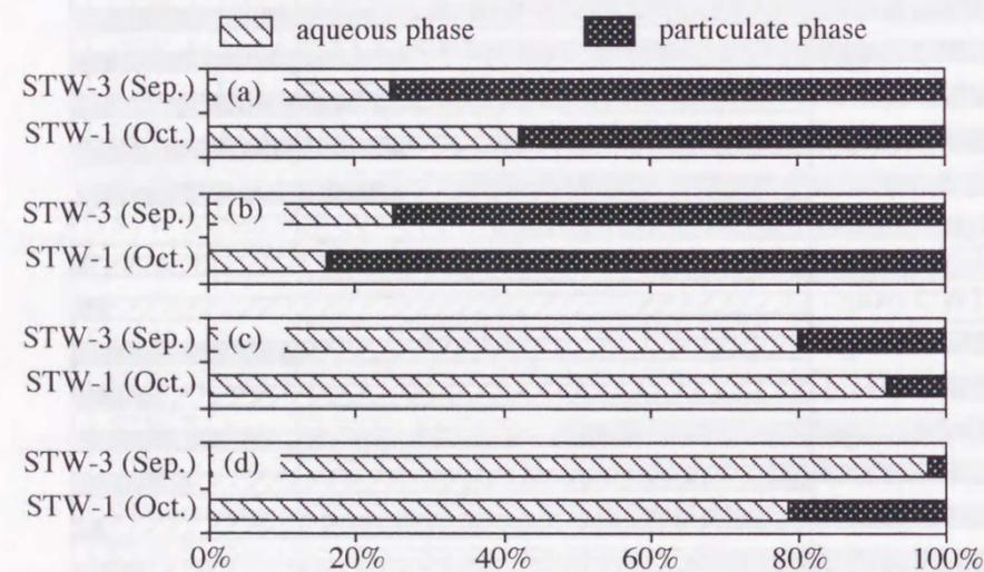
Figure 3.11 Phase distribution of NP1EO in the influent (a), primary effluent (b), secondary effluent (c) and final effluent (d) from STPs in 2000.
