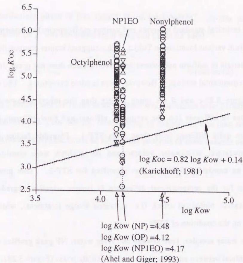
**Figure 3.27** Relationship between octanol-water partition coefficients ( $K_{ow}$ ) and organic carbon-water partition coefficients in the environmental samples ( $K'_{oc}$ ).
