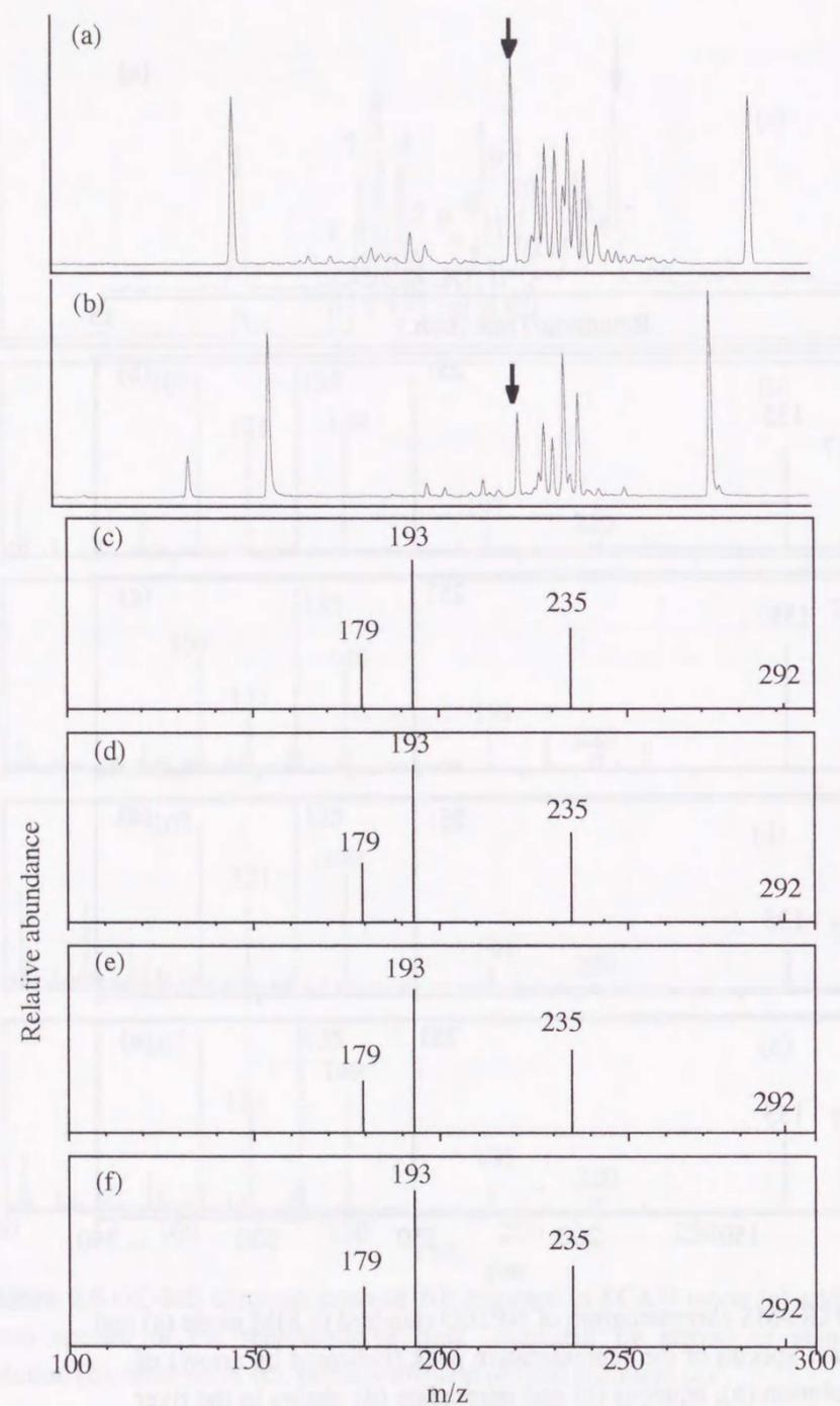
**Figure 2.10** GC-MS chromatogram of NP1EC standard (a) and river water (b) in SIM mode and methylated NP1EC mass spectra of representative peak (indicated by arrow) of standard solution (c), final effluent (d), river water (e) and sewage sludge (f).
