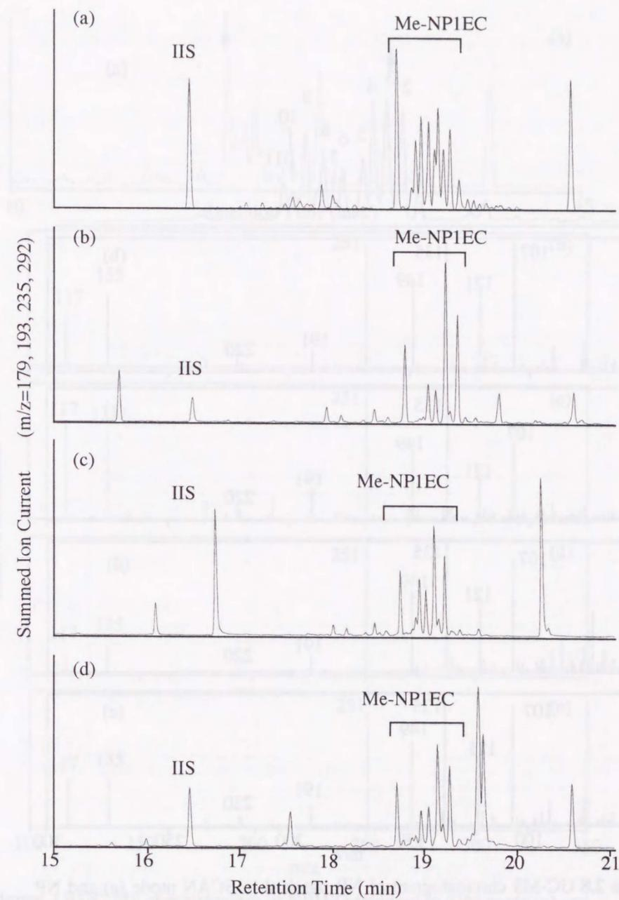
**Figure 2.7** GC-MS chromatograms of methylated NP1EC in SIM mode. Standard (a), sewage effluent (b), river water (c) and activated sludge (d). Standard Me-NP1EC; methylated NP1EC, IIS; anthracene-*d*10.
