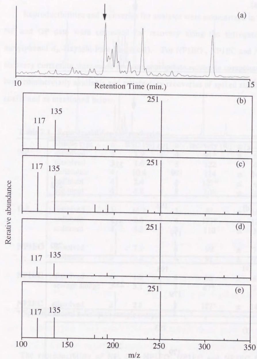
**Figure 2.9** GC-MS chromatogram of NP1EO standard in SIM mode (a) and NP1EO mass spectra of the representative peak (indicated by arrow) of standard solution (b), aqueous (c) and particulate (d) phases in the river water and sediment (e).
