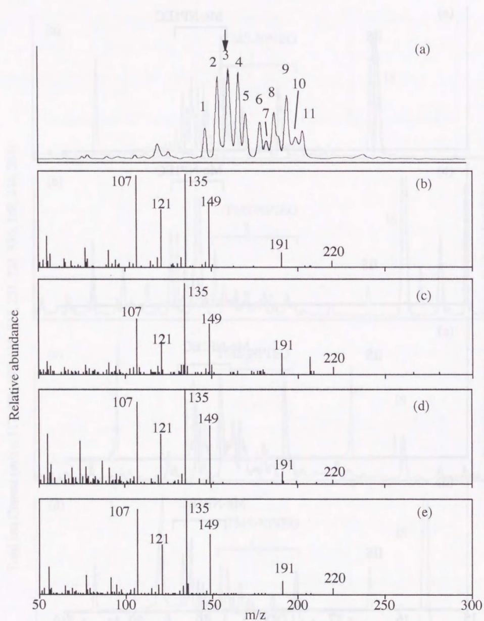
**Figure 2.8** GC-MS chromatogram of NP standard in SCAN mode (a) and NP mass spectra of the representative peak (indicated by arrow) of standard solution (b), river water (c), primary effluent (d) and sediment (e).
