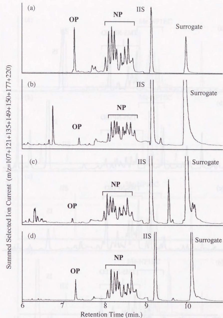
**Figure 2.5.** GC-MS chromatogram of NP and OP in SIM mode. Standard solution (a), aqueous (b) and particulate (c) phases in the river water and sediment (d) samples. IIS; anthracene-*d*10, Surrogate; 4-*n*-NP-*d*4.
