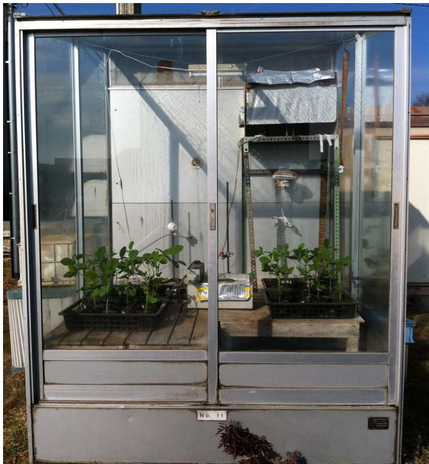
Fig. 3.3.1. Phytotrons and control room were used for exposure of plants
