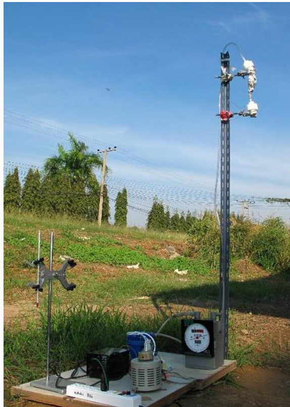
Fig.2.3.9. Measurement tower in Nakhon Pathom measurement site
