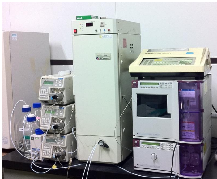
Fig. 2.3.13. HPLC system for peroxides measurement
