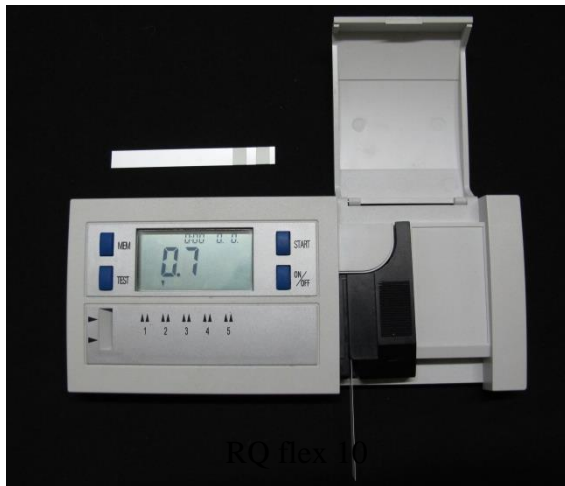
Fig. 2.3.12. RQ flex 10 system for peroxides measurement
