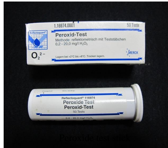
Fig. 2.3.12. RQ flex 10 system for peroxides measurement
