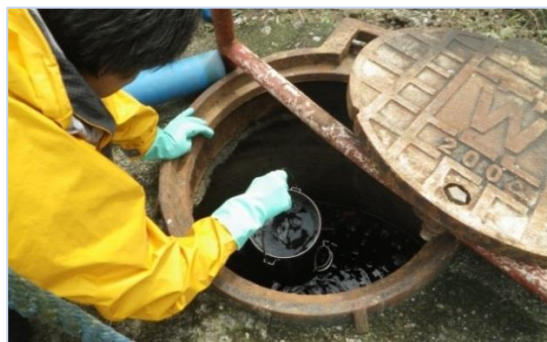
Grab sampling of leachate from a tank
