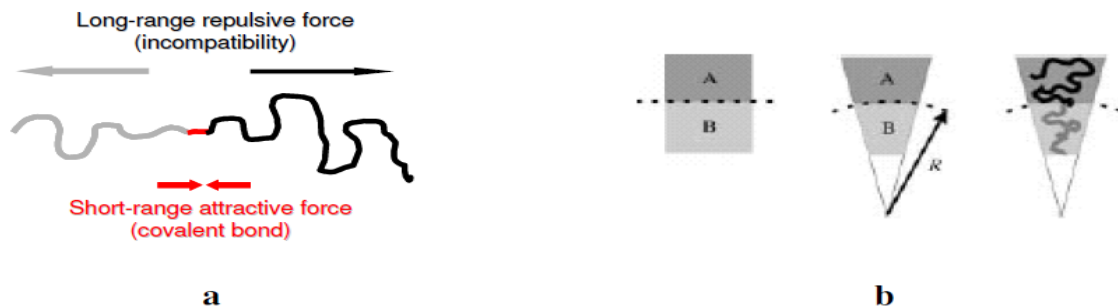
Figure A-1-5.a): Schematic representation of two simultaneously present interactions leading to the self-organisation of block copolymers. b): Local geometry and the curvature of domains and interfaces: A, B – domains; R – curvature radius of the interface (for a planar interface R = \infty ) [29].
