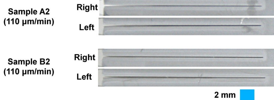
Fig. 2.16: Summary of the kerfloss obtained in the two electrolyte flow modes. Bi-directional flow shows a strong increase in the kerfloss homogeneity between the two opposite face of the silicon ingot.
