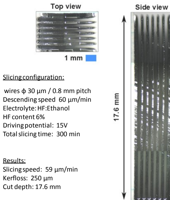
Fig. 2.17: Demonstration of a slicing experiment realized in potentiostatic mode.
