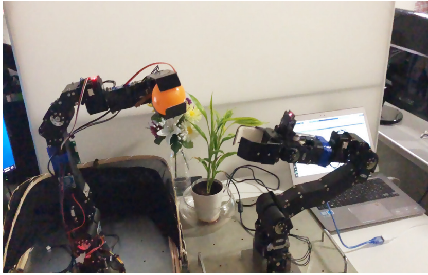
Figure 3.5: Robot arms controlled by MATLAB
