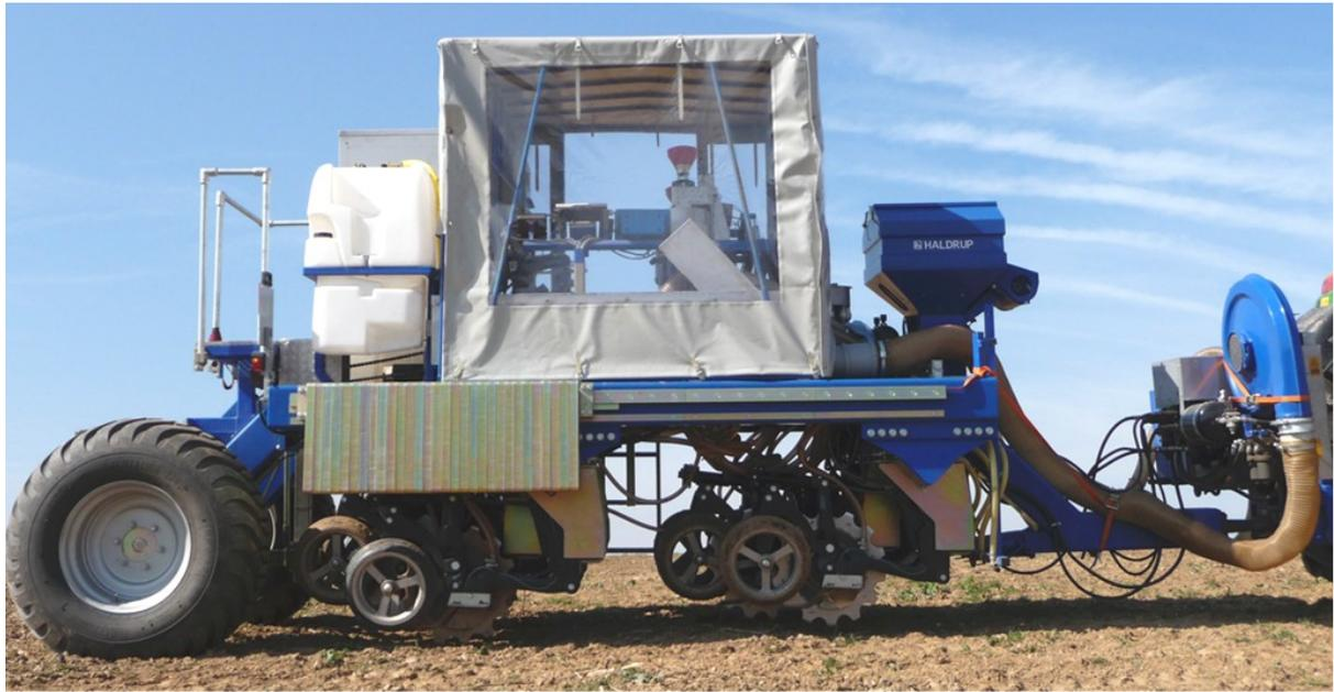
Fig. A 1. Prototype plot seeder with cross-slot openers.
